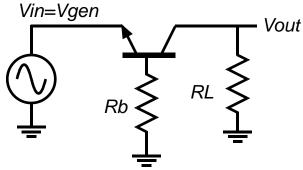
Above is the AC small signal representation of transistor circuit.
