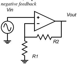
The amplifier has a differential gain of  $2 \cdot 10^7$ . R1=1 kOhm, R2=19 kOhm. The op-amp has infinite differential input impedance and zero differential output impedance.
