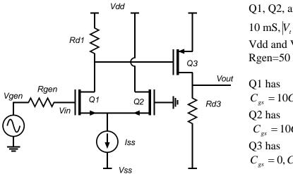
Q1, Q2, and Q3 have  $v_{sat}c_{ox}W_g =$ 10 mS,  $|V_t| = 0.5$  volts, and  $\lambda = 0$  V<sup>-1</sup>. Vdd and Vss are +/- 3.3 Volts. Rgen=50 kOhm and Iss=2 mA.
