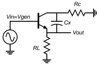
Above is the AC small signal representation of transistor circuit. Rc= 2000 Ohms. RL= 10,000 Ohms. The transistor is biased at 2 mA DC emitter current, so that re=13Ohms.  $C_x = 20$  fF
