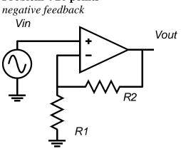
The amplifier has a differential gain of  $4 \cdot 10^5$ . R1=1 kOhm, R2=39 kOhm. The op-amp has infinite differential input impedance and zero differential output impedance.
