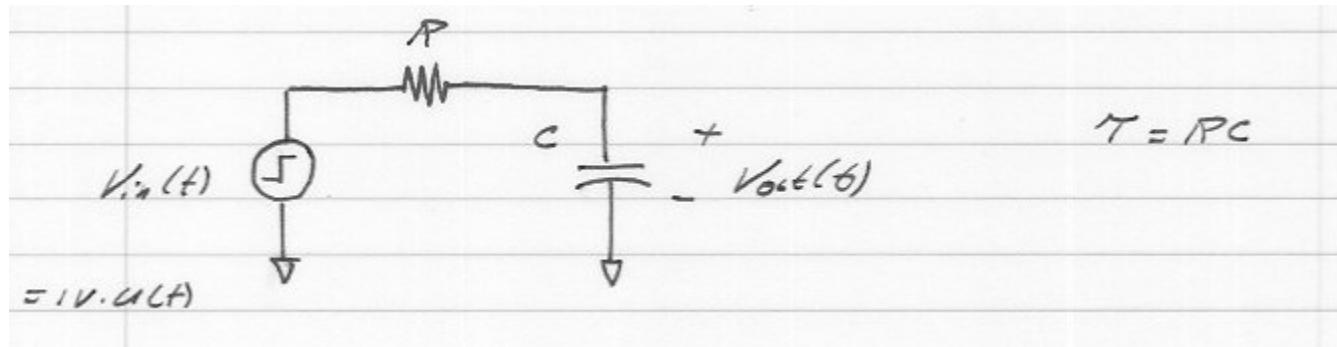
$$v_i(t) = v_o(t) + \gamma \frac{\partial v_o(t)}{\partial t}$$
