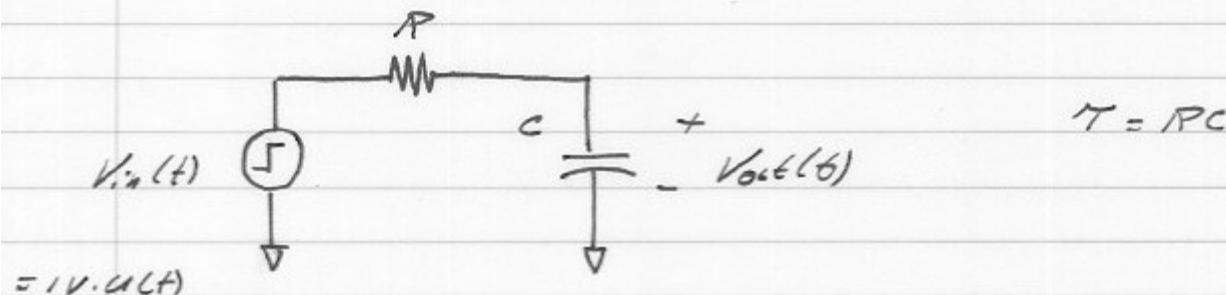
How do we solve for  $V_{out}(t)$  given  $V_{in}(t)$ ?
