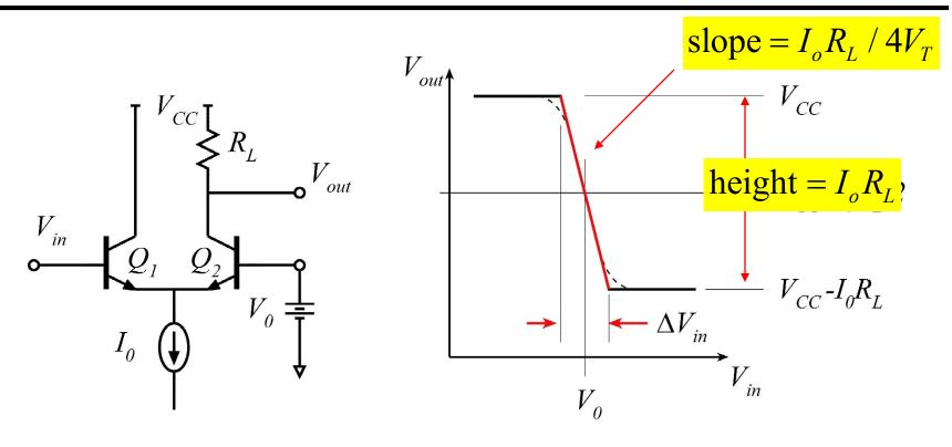
so, the slope of the switching region is  $I_o R_L / 4V_T$ , while the output voltage swing is  $I_o R_L$ ,
