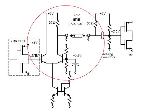
One example of this: the digital  $50\Omega$  coaxial cable interface between the PRBS pulse generator and the LED/laser driver in lab project choice #2.
