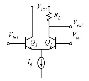
You can repeat this calculation for a differential input  $\rightarrow$  different  $\Delta V_{in}$
