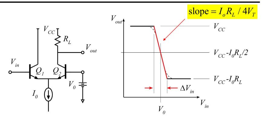
DC bias  $V_{in}$  at zero Volts, then apply a small signal: what is the gain ?  $g_m = g_{m1} = g_{m2} = I_o / 2V_T$ ,  $A_v = \partial V_{out} / \partial V_{in} = g_m R_L / 2 = I_o R_L / 4V_T$
