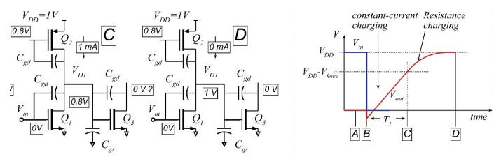
Switching time between C and D: 2nd part: charging from 0.8V towards 1V
