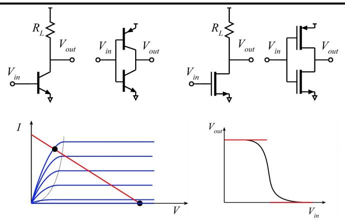
In these common-source-like and common-emitter-like circuits either or both  $V_{out,high}$  and  $V_{out,low}$  are set by saturation.
