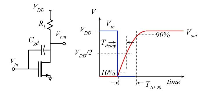
The input voltage falls suddenly, turning the FET off. Node is charged through resistance *R*; charging is exponential Equivalent capacitance  $C = \Delta Q / \Delta V$ , time constant  $\tau = RC$  $T_{rise/fall} = 2.2\tau$  and  $T_{delay} = \tau \ln(2)$
