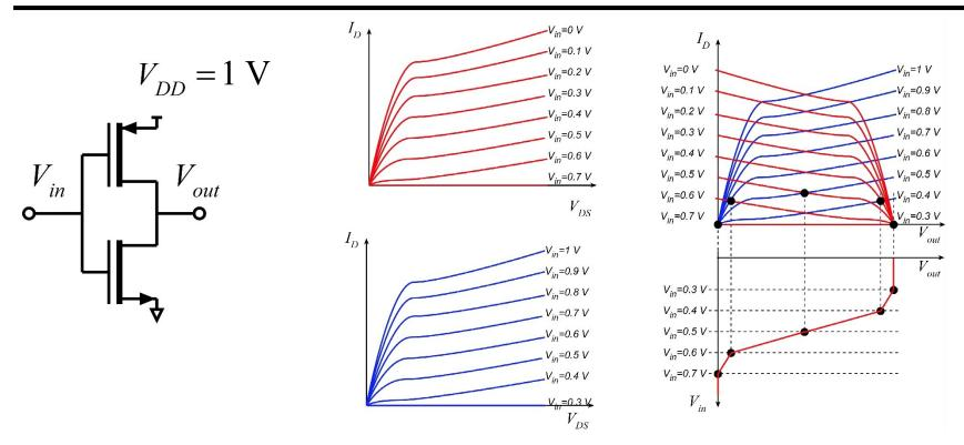
$I_{D,NFET} = I_{D,PFET}$  and  $V_{DS,PFET} = V_{DD} - V_{DS,NFET}$
