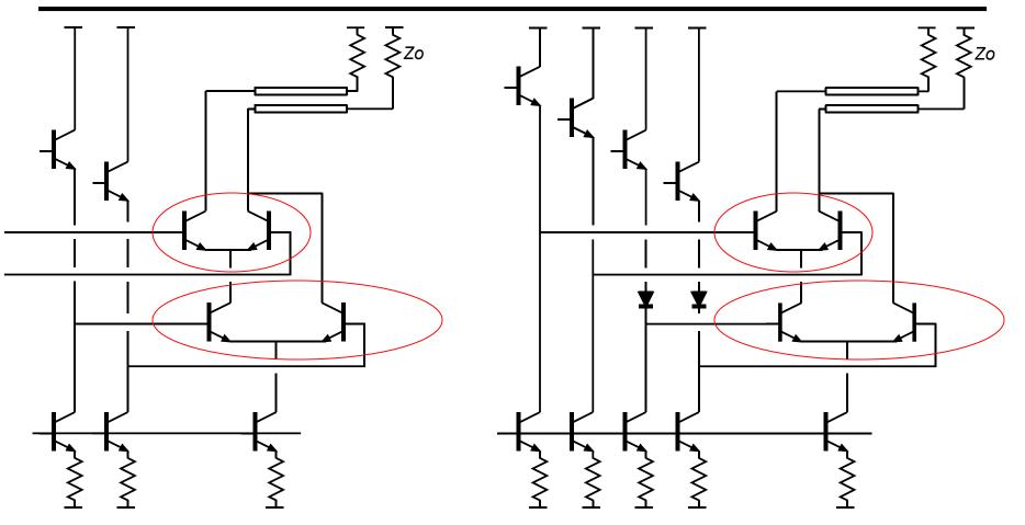
There are also logic families using bipolar differential pairs, current mode logic, left, and emitter coupled logic, right
