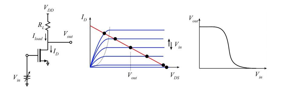
Here, the lower limit on  $V_{out}$  is set by saturation, and the upper limit by cutoff
