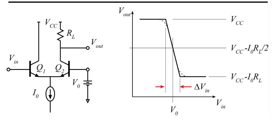
The stated levels on the diagram are easily found. But, how do we find  $\Delta V_{in}$ ?
