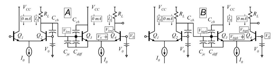
Let us calculate the risetime at the base of Q3 Times are relative to the time at which the collector current of Q2 switches to zero.
