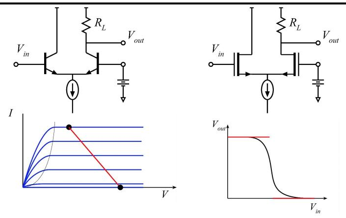
We can design differential current-steering circuits such that both  $V_{out,high}$  and  $V_{out,low}$  are set by cutoff.
