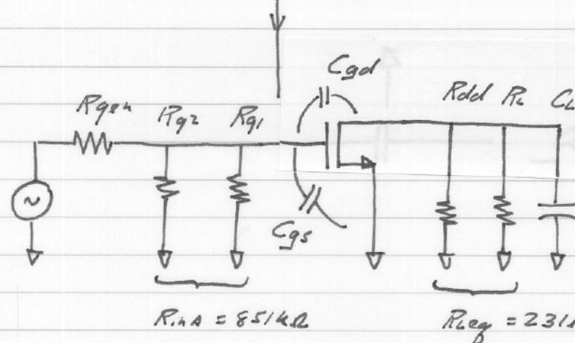
$$R_i = R_{gen} // R_{inA} = 9.9 \text{ k}\Omega$$
