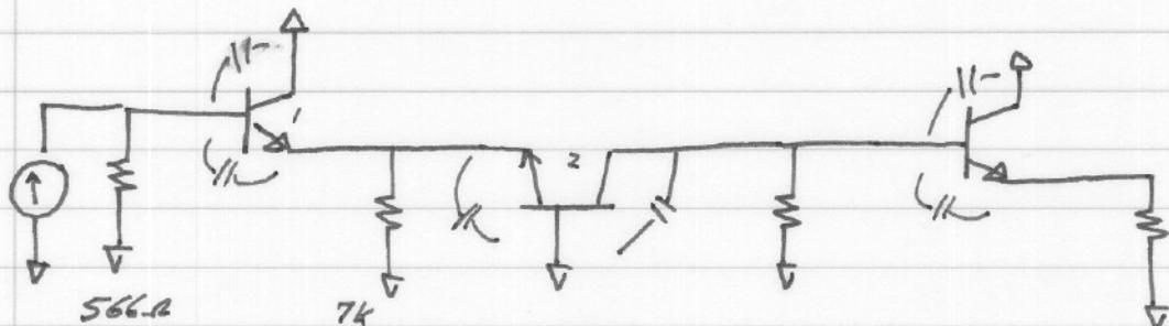
Replace each capacitor not-to-ground with a Miller capacitor  $C(1-A) = C_{Miller}$ .
