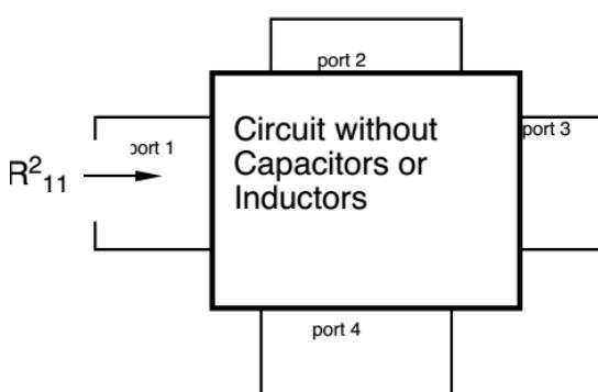
$$\frac{V_{out}}{V_{gen}} = \left( \frac{V_{out}}{V_{gen}} \right)_{MB} \frac{1 + b_1s + b_2s^2 + \dots}{1 + a_1s + a_2s^2 + \dots}$$
