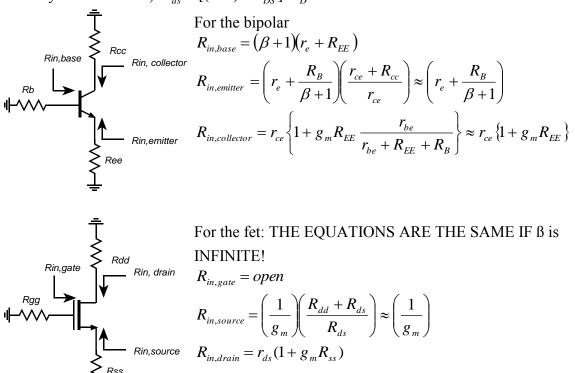
Be warned that in the equations above Rcc, REE and RB are the equivalent resistances seen by the transistor. So in, the amplifier circuits below, THINK: "what is the effective resistance seen by the transistor?", before plugging into the equations.
