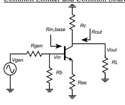
$$R_{in} = R_B \| R_{in,base} = R_B \| (\beta + 1)(R_{EE} + r_e)$$
