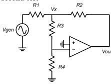
Use this circuit when you need to measured the low-frequency open-loop gain of an op-amp. Make R1=R2=10 kOhm. Lets leave R3 and R4 unspecified for a moment.
