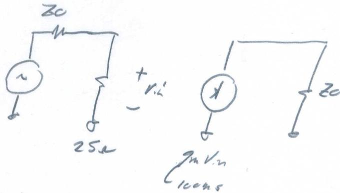
$$= 2 \cdot \frac{25}{25+50} \cdot \frac{(-g_m Z_0)}{\frac{100 \text{ mS}}{50 \text{ ohm}}} = \frac{25}{75} \cdot \frac{-100 \text{ mS}}{50 \text{ ohm}} = -\frac{10}{3}$$
