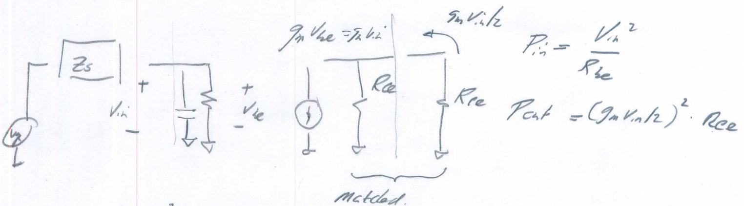
$$\frac{P_{out}}{P_{in}} = \frac{(g_m/2)^2 R_{ce}}{1/R_{be}} = \frac{g_m^2}{4} R_{ce} R_{be} = \frac{(0.1S)^2}{4} 1k\Omega \cdot 10k\Omega = \underline{\underline{25,000}}$$
