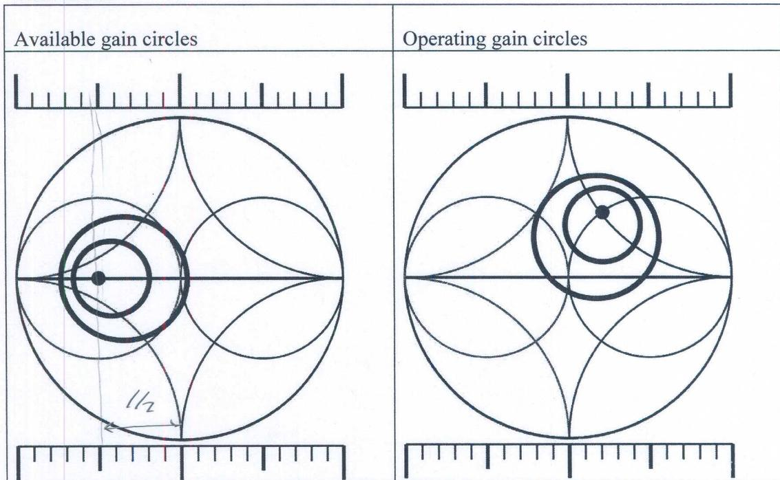
At 10 GHz, a MOSFET in common-source mode operating and available gain circles as shown. Find the optimum generator and load impedances (in complex Ohms).
