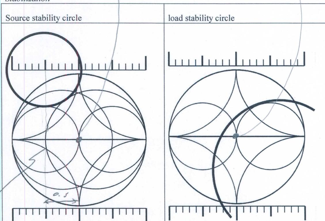
A MOSFET in common-source mode has  $S_{11} = 0.5$  and  $S_{22} = 0.3$ . Source and load stability circles are as shown. Draw \*\*\*3\*\*\* circuit diagrams, giving resistor values, of methods of stabilizing the transistor.
