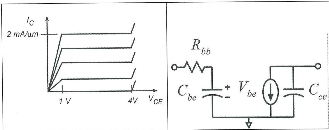
An HBT has the output characteristics as shown, with a maximum 2mA/micron collector current. The (somewhat contrived) device model is to the right, with
