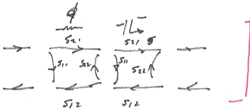
$$2 \left[ S_{21}^{\text{overall}} = \frac{S_{21}^R S_{21}^{T^*}}{1 - S_{22}^R S_{11}^{T^*}} = \frac{(4/5)(5)}{1 - (1/5)(0.5)} \right. \\ \left. = \frac{4}{1 - 0.1} = 4.44 \quad \text{half for formula} \right. \\ \left. \text{half for meth.} \right]$$
