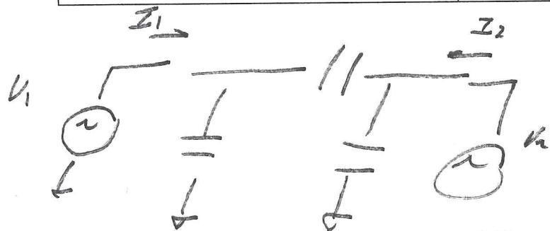
$$\Rightarrow \text{connection: } [Y_{ij}] = \begin{bmatrix} j\omega C_{11} + j\omega C_{12} & -j\omega C_{12} \\ -j\omega C_{12} & j\omega C_{22} + j\omega C_{12} \end{bmatrix}$$
