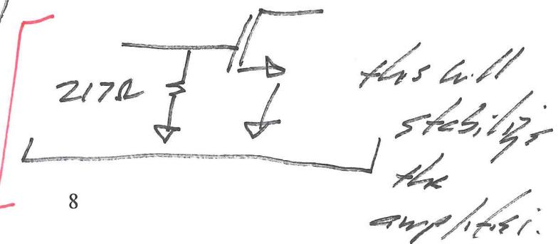
$$S_{11} = 0, \quad S_{12} = Q_1, \quad S_{21} = \delta, \quad S_{22} = 0.5$$
