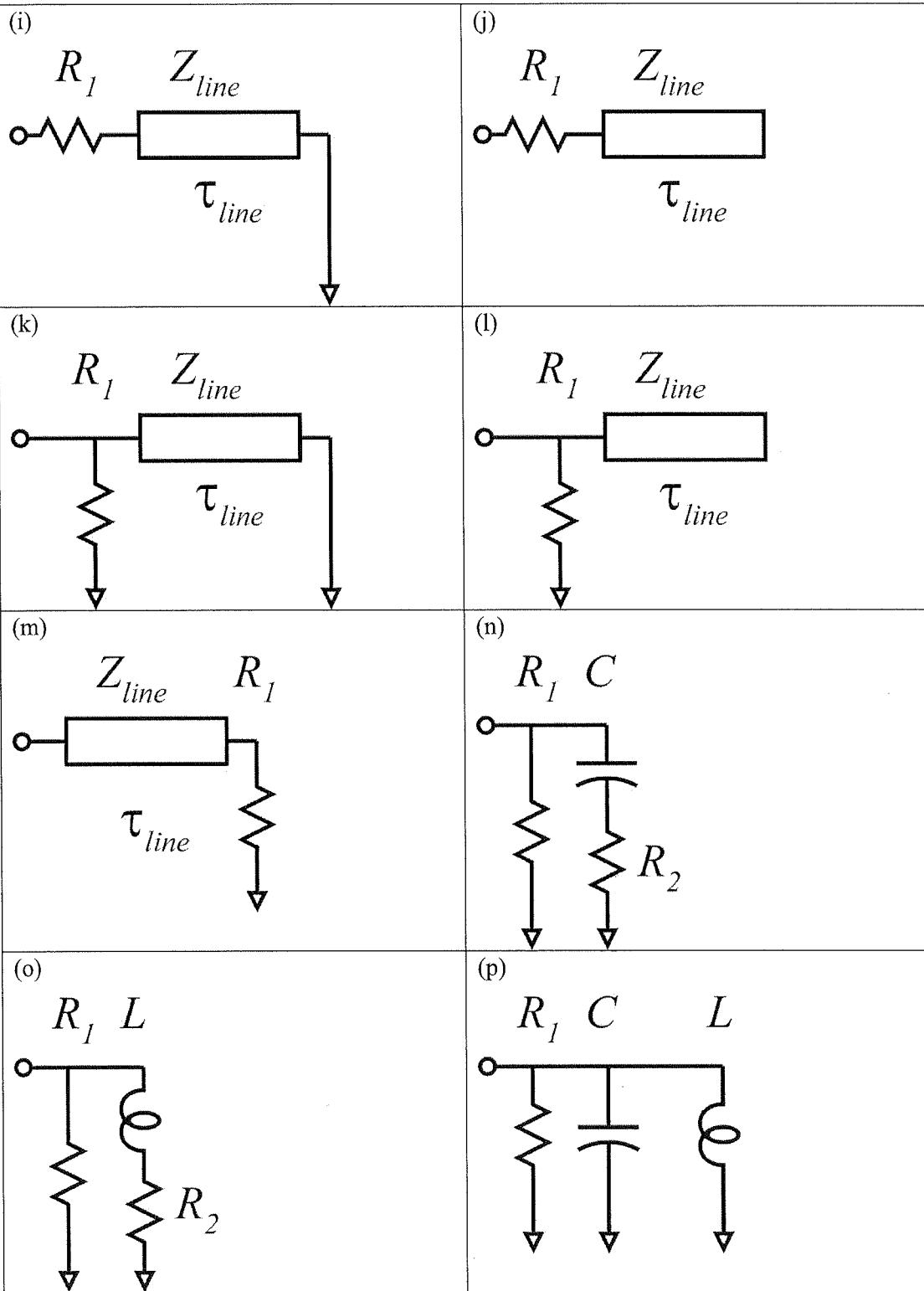
First match each Smith Chart with each circuit. ***Then determine as many component values as is possible*** (RLC values, transmission line delays and characteristic impedances)...note that some values cannot be determined with the information given. The charts all use 50 Ohm normalization:
