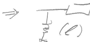
$R_L = 93\Omega$ ,  $Z_0$  unknown. line is  $1/4 @ 16\text{GHz}$ .
