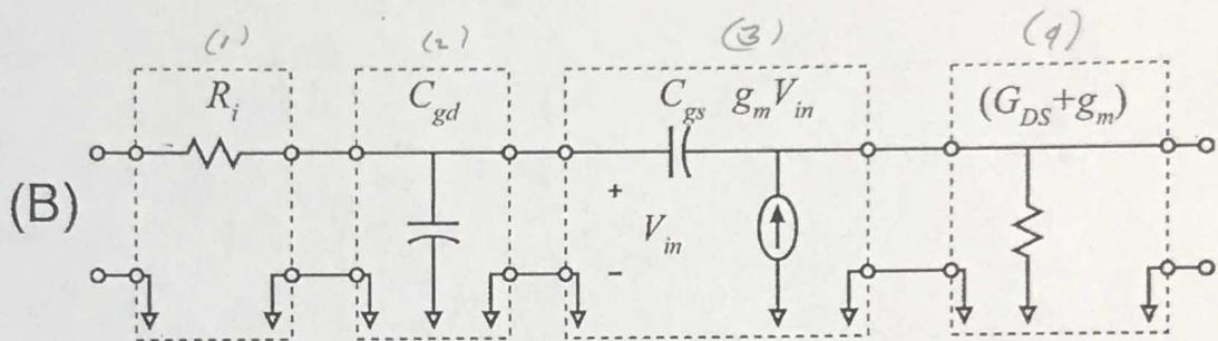
The network (A), which represents the hybrid-pi FET model in source-follower operation, can be represented as the cascaded network (B) below.
