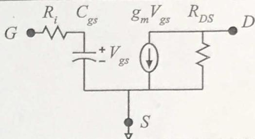
$$Y_{11} = \frac{1}{R_i + j\omega C_{gs}} = \frac{1}{50\Omega - j50\Omega}$$
