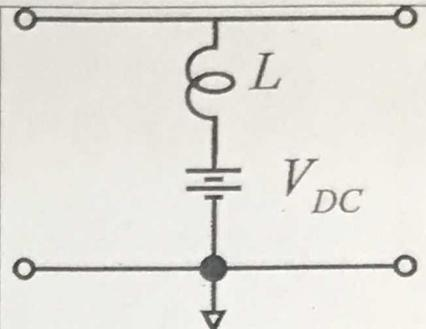
$$\text{Minimum value of } L \text{ to meet } S_{21} \text{ specification} = \frac{4 \text{ nH}}{400 \text{ nA}}$$
