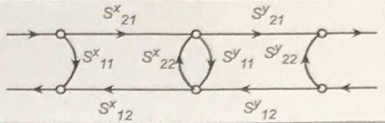
$$S_{21}^Z = \frac{S_{21}^X S_{21}^Y}{1 - S_{22}^X S_{11}^Y}, \quad S_{12}^Z = \underline{\hspace{10em}}$$
