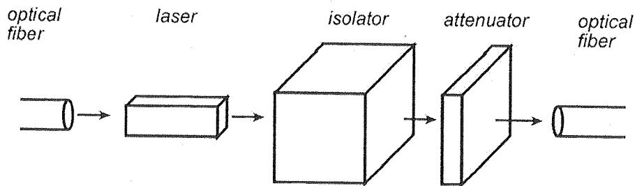
A laser (more precisely, a semiconductor optical amplifier) is coupled to an isolator and an attenuator to help stabilize it. Defining port 1 on the left and port 2 on the right, we have
