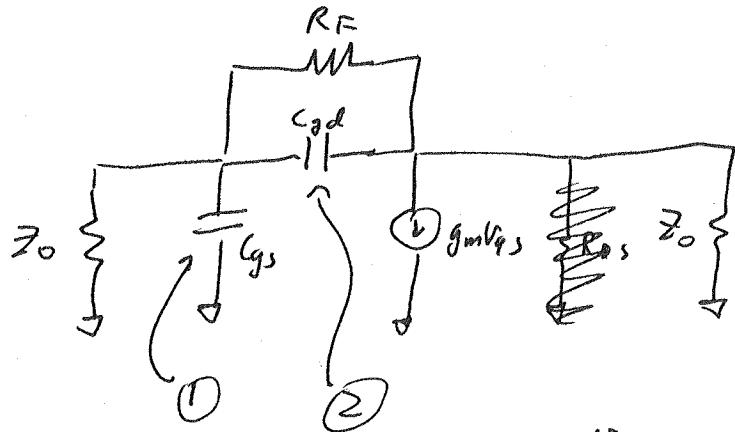
$$R_{11}^o = Z_o \parallel \underbrace{\frac{R_F}{1+A_v}}_{Z_o \text{ by definition}} = 25 \Omega$$
