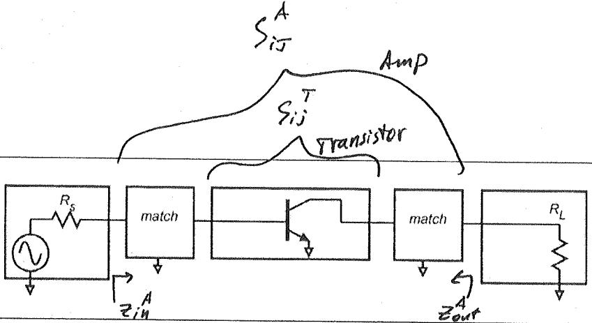
Matching networks are then designed which *Match the amplifier input to a 25 Ohm load and a 150 Ohm generator.*
