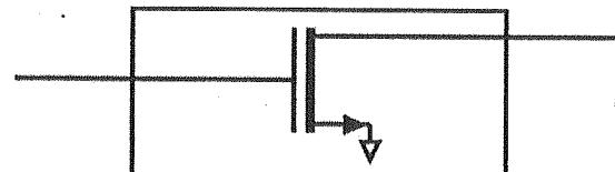
If necessary, the transistor is stabilized. It is then matched on input and output to 50 Ohm source and load. What transducer power gain is then obtained?
