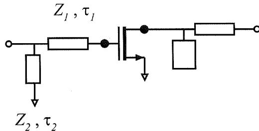
The shunt line #2 must have 50 Ohm characteristic impedance and is 0.1 (guide) wavelength long at the design frequency.
