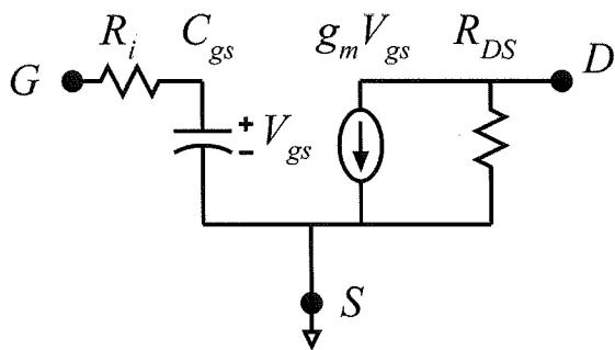
$$S_{11} : \left[ \begin{array}{l} Z_{11} = R_i + 1/(j\omega C_{gs}) \\ Z_{11}Z_0 = R_i Z_0 + 1/(j\omega C_{gs} Z_0) \end{array} \right] \quad \left. \right\} \quad (2)$$
