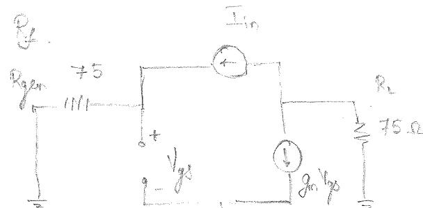
$$R_{22} = R_f || R_{in} \quad (\text{Now add } R_f \text{ back again})$$
