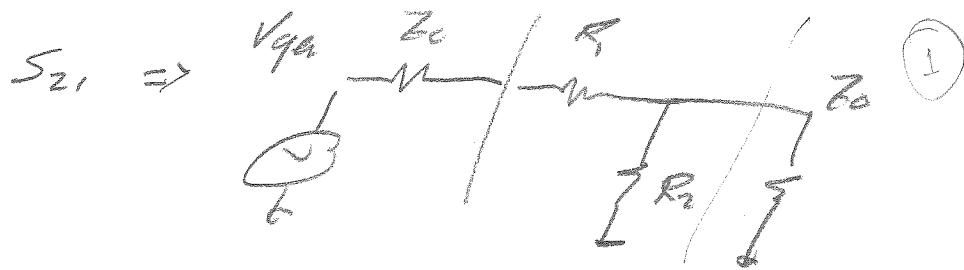
$$S_{21} = \frac{2 \frac{V_o}{V_{gds}} / \frac{Z_0}{Z_0 + Z_0 = Z_{gds}}}{(Z_0 \parallel R_2) + R_1 + Z_0} = \frac{(Z_0 \parallel R_2) \parallel Z_0}{(Z_0 \parallel R_2) + R_1 + Z_0}$$
