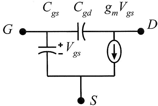
A FET has a transconductance of 1 mS per micron of gate width.  $C_{gs}$  is 1 fF per micron of gate width, and  $C_{gd}$  is 0.1 fF per micron of gate width
