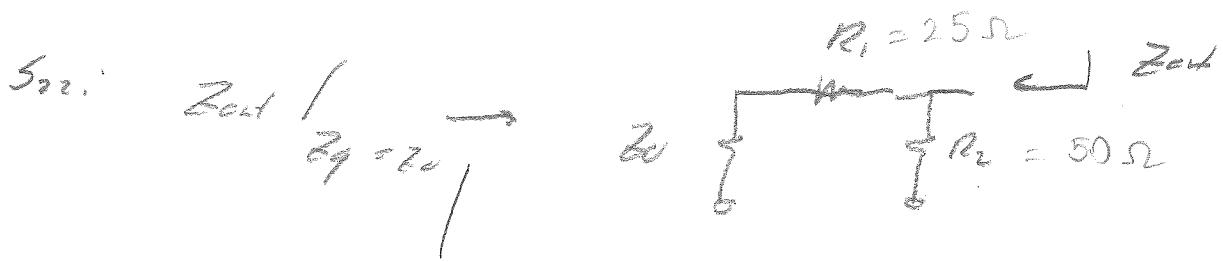
$$= R_2 \parallel (R_1 + Z_0) = 50 \Omega \parallel 75 \Omega = 30 \Omega$$
