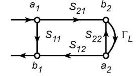
$$T = \frac{b_1}{a_1} = \Gamma_{in} = \frac{S_{11}[1 - S_{22}\Gamma_L] + S_{21}\Gamma_L S_{12}}{1 - S_{22}\Gamma_L}$$
