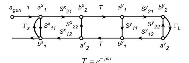
The signal flow graph compactly and visually represents the many equations describing the system.
