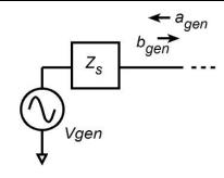
$$b_{gen} = T_s V_{gen} / \sqrt{Z_0} + \Gamma_s a_{gen}$$
