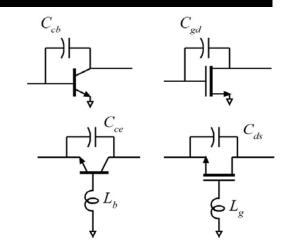
Some of these are device parasitics, some arise only from poor interconnect design near the device terminals.
