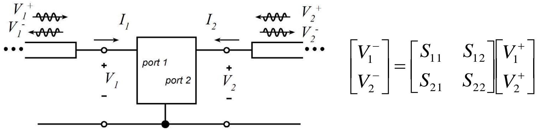
At port 1,  $V_1 = V_1^+ + V_1^-$  and  $I_1 = (V_1^+ - V_1^-)/Z_0$
