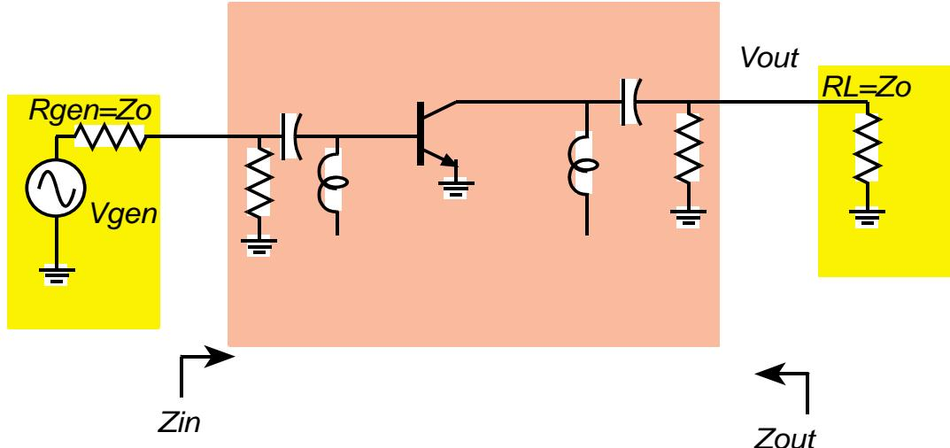
S11 and S22 can be directly related to input and output impedances
