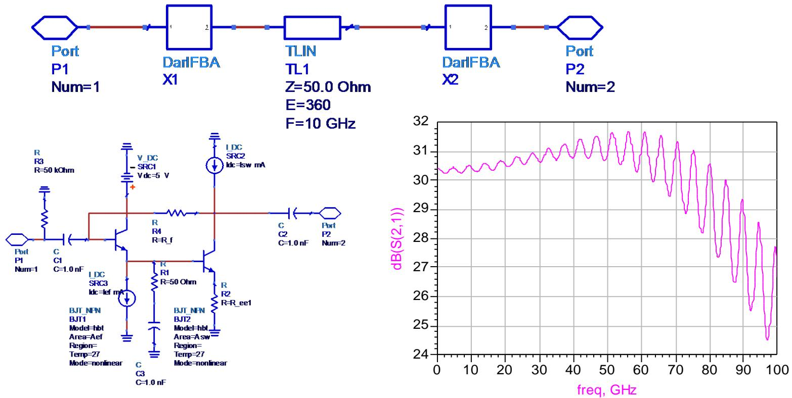
Standing waves on transmission lines cause gain/phase ripples of the form  $(1 - \Gamma_s \Gamma_L \exp(-j2f\tau))^{-1}$ . Either we must have short transmission lines, or the lines must be well-terminated
