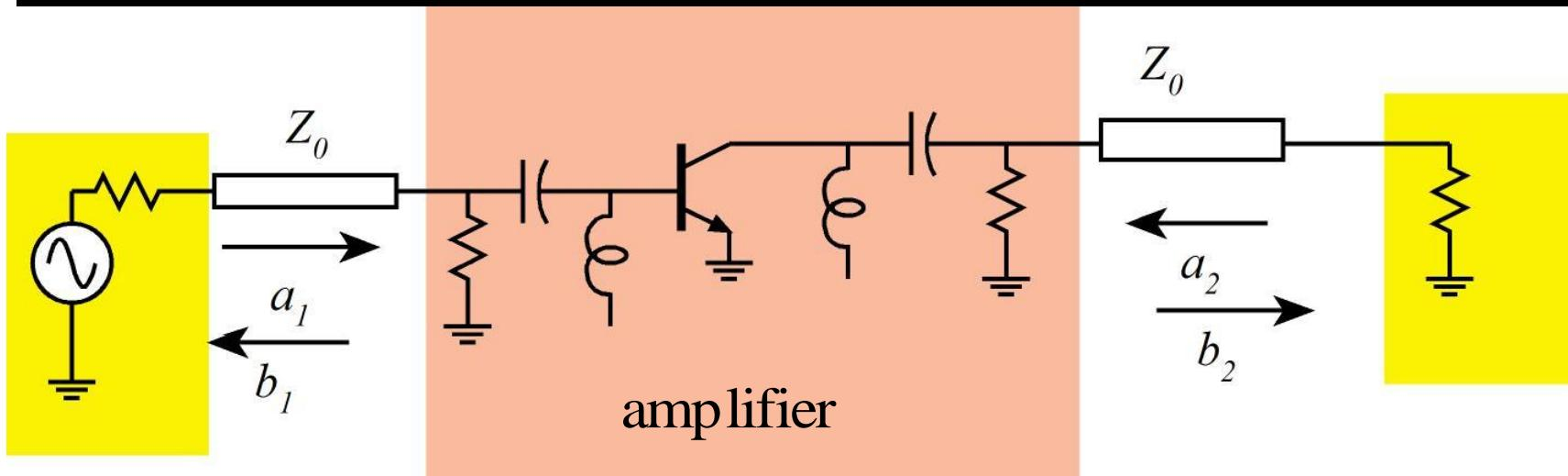
S - parameters are rigorously defined in terms of the wave amplitudes on transmission lines connected to the device under test :
