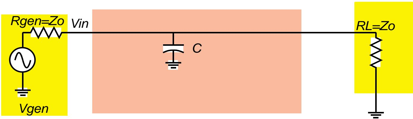
$$S_{21} = \frac{\left( Z_o \parallel \frac{1}{j\omega C} \right)}{Z_0 + \left( Z_o \parallel \frac{1}{j\omega C} \right)} = S_{12} = \frac{1}{1 + j\omega C Z_0 / 2}$$
