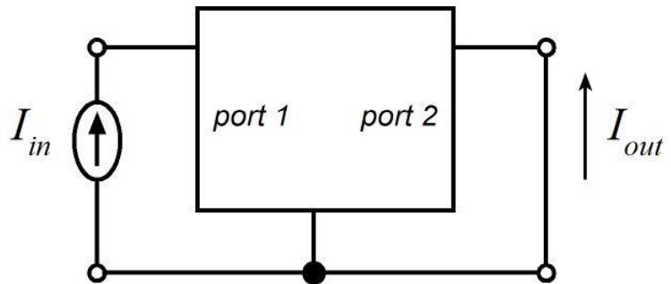
$$\frac{I_{out}}{I_{in}} \Big|_{\text{output short-circuited}} = h_{21}$$
