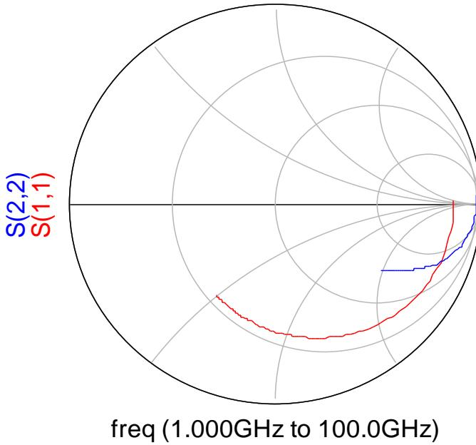
$$S_{11} = \frac{(Z_{in}/Z_0) - 1}{(Z_{in}/Z_0) + 1}, \text{ where } Z_{in} = Z_{in} \Big|_{Z_{load}=Z_0}$$
