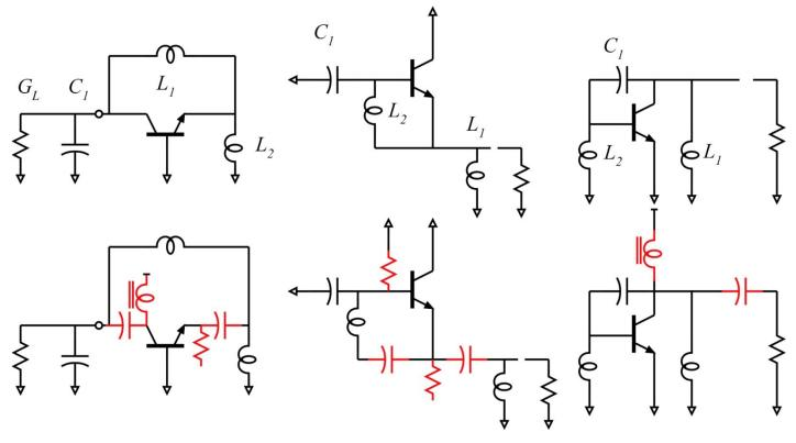
The AC small-signal network is shown above in common - (base, collector, emitter) form. Feeback is through inductors  $L_1$  and  $L_2$ .
