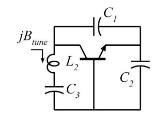
Replace with the series combination  $L_2$  and  $C_3$ .
