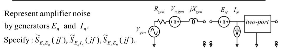
Represent generator noise by generators  $V_{gen}$  (signal) and  $V_{n,gen}$  (noise).
