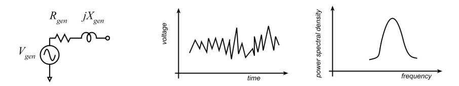
The generator signal voltage has some power spectral density  $\widetilde{S}_{V_{gen}V_{gen}}(jf)$ , having units of  $(V^2/Hz)$ .
