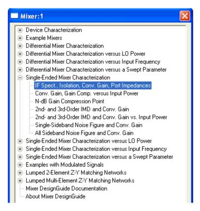
You will find a large selection of mixer characterization templates and example mixers. These are grouped according to differential or single-ended mixer interfaces. Within each group, you will find 4 categories of measurements, all using the harmonic balance simulation mode.
