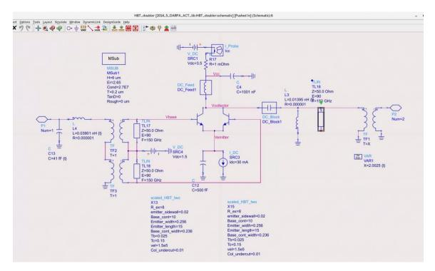
The circuit has a bias feed line DC\_Feed1, a blocking capacitor DC\_block1, and an output ideal tuning network L3 and TF1. There is also an open-circuited line that is a quarter wavelength at the input frequency. This short-circuits the input frequency and its third harmonic at the output, while presenting an open at the 2nd harmonic.
