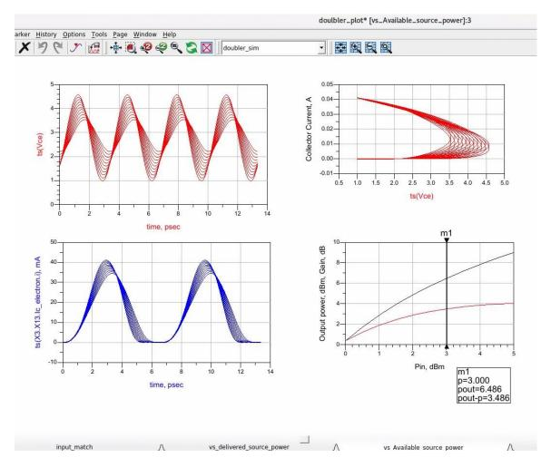
Note the nearly ideal frequency doubler load line in the top righthand corner. This plot shows power added efficiency versus Available input power. Once again there is also a tab which will show a graph of output power and efficiency versus delivered source power. There is also a tab for large signal input match.
