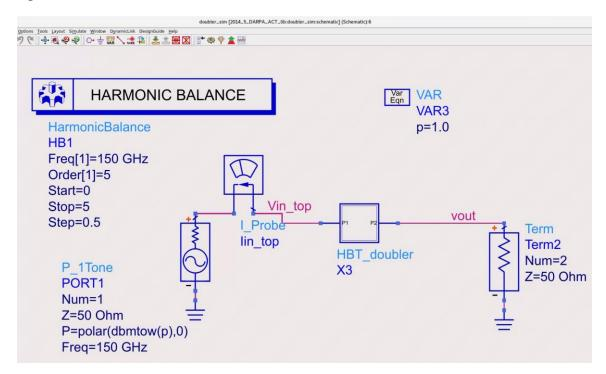
THis drives a frequency doubler at 150 GHz input frequency.
