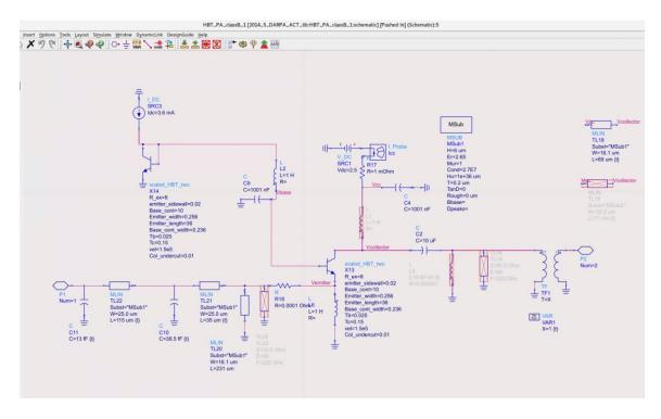
The circuit has a bias feed line TL19, and , crossed out, and ideal output tuning network consisting of L3 and TF1. Also crossed out is 1/4 wavelength transmission line TL16 Which is used to short circuit the second harmonic of the output signal.
