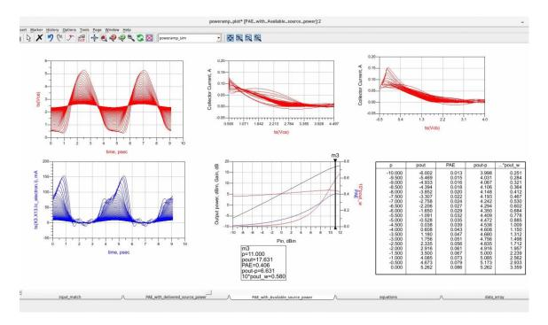
Note the class B loadline. Note the plot of output power and PEA vs. Available input power. Note also the other graph tab that gives plots of PA versus \*delivered\* (as opposed to available) input power; this is useful to simulate the performance of the PA as a function of the output tuning network, when the \*input\* tuning network has not yet been correctly adjusted.
