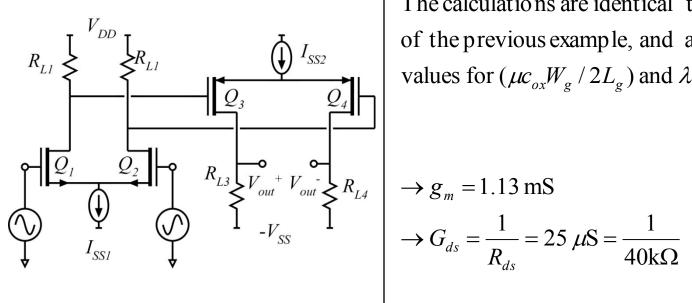
The calculations are identical to those of the previous example, and all FETs have the same values for  $(\mu c_{ox}W_g/2L_g)$  and  $\lambda$ .
