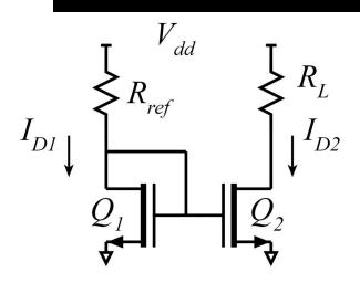
If the  $(1 + \lambda V_{DS})$  term is small, mirror provides nearly constant current over a wide range of load resistances, i.e. over a wide range of voltages.
