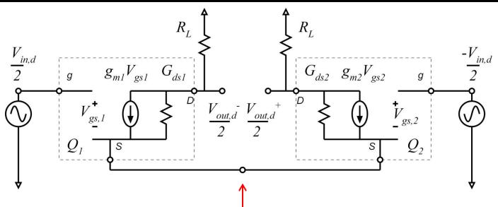
From symmetry, the small - signal voltage at this point must be zero.
