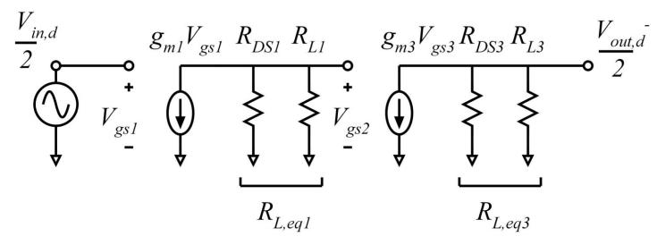
Replace transistor symbols with small - signal models
