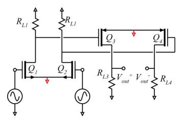
In the small signal diagram at left, the supply votages have been replaced by short-circuits, the supplycurrents have been replaced by open-circuits, but the transistors have not yet been replaced by their small-signal models.
