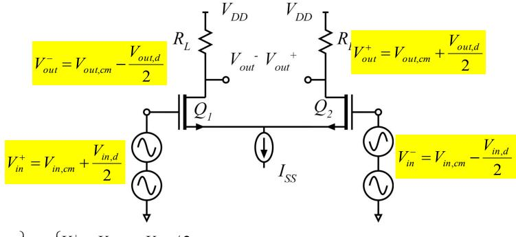
$$\begin{aligned} V_{in,d} &= V_{in}^{+} - V_{in}^{-} \\ V_{in,cm} &= (V_{in}^{+} - V_{in}^{-})/2 \end{aligned} \longleftrightarrow \begin{cases} V_{in}^{+} &= V_{in,cm} + V_{in,d}/2 \\ V_{in}^{-} &= V_{in,cm} - V_{in,d}/2 \end{aligned}$$
