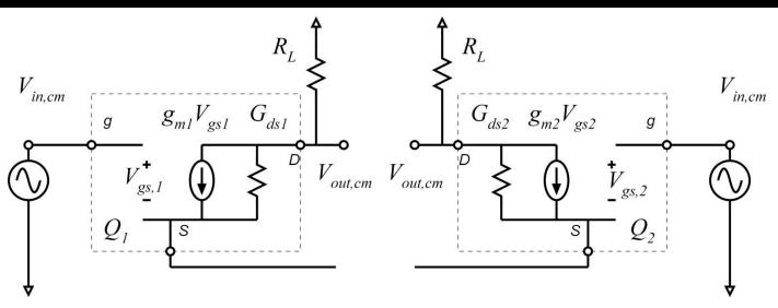
From symmetry, all the voltages on the right side are \* the same as \* those on the left ... and, the virtual open has broken the connection between the 2 sides of the circuit
