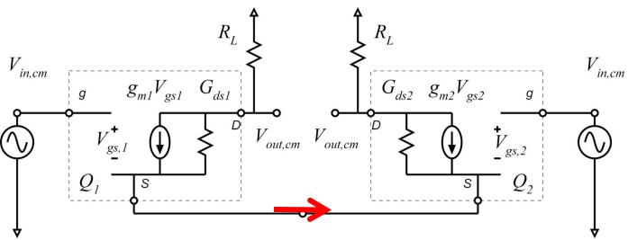
From symmetry, the small - signal current in this wire must be zero.
