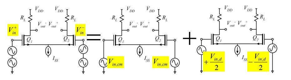
The  $(V_{in}^+, V_{in}^-)$  inputs can always be written as a superposition of  $V_d$  and  $V_{cm}$ . So , analyze the circuit for \* differential \* and \* common - mode \* gain.
