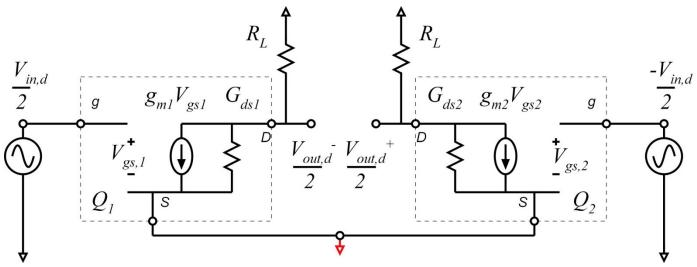
From symmetry, all the voltages on the right side are negatives of those on the left ... and, the virtual ground has broken the connection between the 2 sides of the circuit
