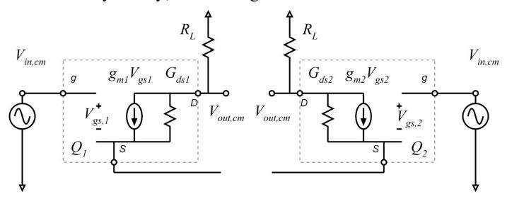
So, it makes no difference if we cut this wire. This (should be) called a virtual open.
