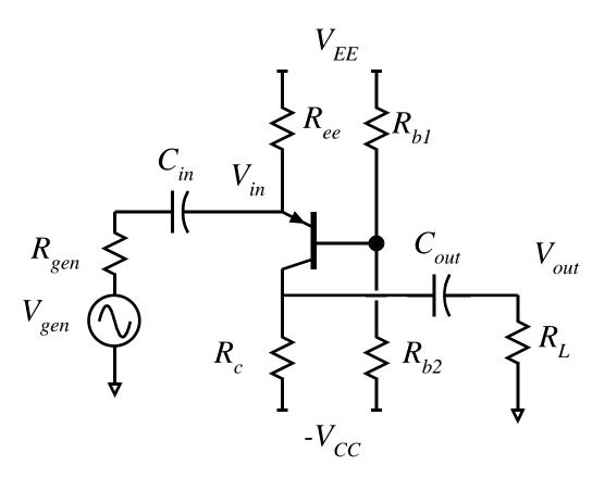
On the circuit diagram above, label the DC voltages at **ALL nodes** and the DC currents through **ALL resistors**
