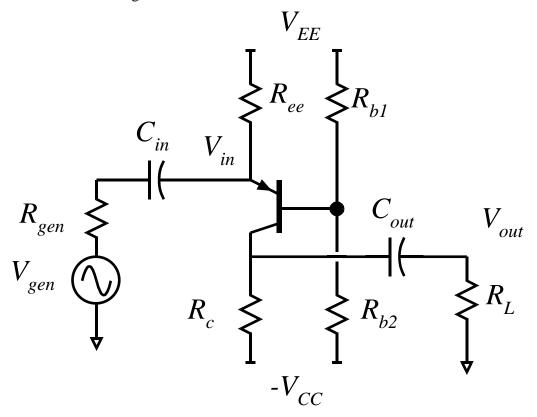
Q1 is a PNP transistor with  $\beta = 100$  and  $V_A = \infty$  Volts. +Vee= +5.0 volts, -Vcc= -5 Volts Cin1 and Cout are very big and have negligible AC impedance. RL=10 kOhm Rgen=100 Ohm,
