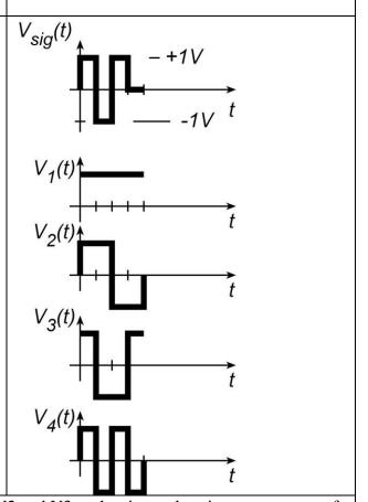
We can view V1 as the DC component, V2 and V3 as the sine and cosine components of the first harmonic, and V4 as the 2nd harmonic
