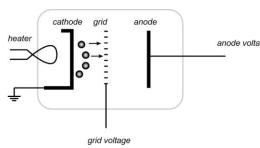
where  $\mu$  is known as the amplification factor and  $k_p$  is a characteristic of the tube having units of amps per volt<sup>3</sup>/2. (a) Defining the output conductance as  $\partial I_a / \partial V_a$  and the
