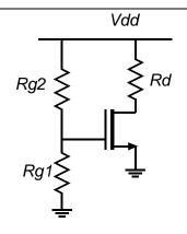
b) Bias stability of the circuit of problem 1(a). <u>First</u>, keeping the same values for Rg1, Rg2, and Rd you found above, compute the drain current and the drain voltage if  $v_{sat}C_{ox}W_g$  is increased to 10%. <u>Second</u>, using the original value  $v_{sat}C_{ox}W_g$ , and keeping the same values for Rg1, Rg2, and Rd you found in 1(a), compute the drain current and the drain voltage if the power supply voltage is increased 10%.
