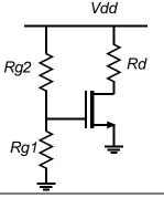
Problem 5: The P MOSFET has a -0.25 V threshold voltage...meaning the gate is 0.25 V negative of the source at the onset of conduction. Use a constant-velocity model:  $v_{sat}C_{ox}W_g = 0.3 \text{ mA/V}.$   $\lambda = 0 \text{ V}^{-1}$
