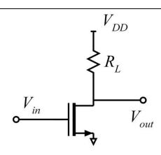
The supply voltage Vdd is 2.0 Volts, and RL is 2kOhm. (a) Graph the common-source characteristics for Vgs=0.3, 0.4, 0.5...1.0 Volts. (b) Add the loadline associated with RL and Vdd to the graph. (c) From this graphs make a separate plot of Vout Vs Vin. What DC input voltage results in an output voltage of 1.0 Volts? (d) from the graph of part c, what is the small-signal voltage gain if the input is biased such that the output is at 1.0 Volts DC?
