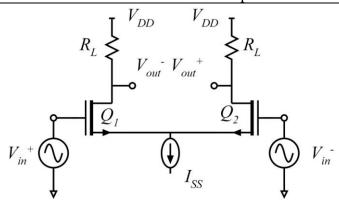
(a) Find  $I_{SS}$  and  $R_L$ . (b) Draw a circuit diagram indicating all DC node voltages and all DC branch currents. (c) Find the transconductance and output conductance of each transistor. (d) Draw a small signal equivalent circuit of each transistor. (e) Draw a small-signal equivalent circuit of the whole amplifier. (f) If  $V_{in}^+ = \text{ImV} \cdot \cos(2\pi \cdot \text{lkHz} \cdot t)$  and
