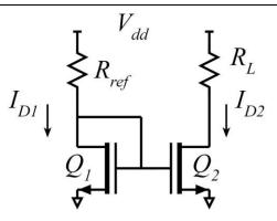
(b) What value is needed for  $W_{g2}$  ? (c) over what range of  $V_{ds2}$ , and over what range of  $R_L$  is the output current  $I_{D2}$  is constant?
