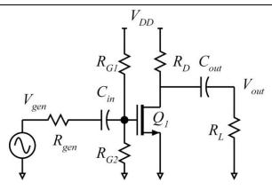
The transistor has  $C_{es} = 0.5$  fF and  $C_{ed} = 0.25$  fF.
