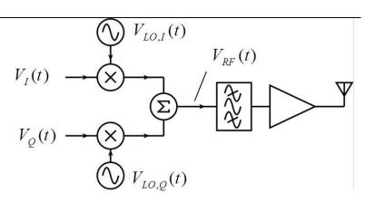
$V_0$  is 0.1 Volts.  $V_I(t)$  is the sum of a 100 mV \*sine\* wave at 1kHz and a 100 mV \*cosine\* wave at 2 kHz.  $V_Q(t)$  is the sum of a 100 mV \*sine\* wave at 3kHz and a 100 mV \*cosine\* wave at 4 kHz. (a) Compute  $V_{RF}(t)$  (b) Compute the Fourier Transform of  $V_{RF}(t)$ . Note carefully the phases of the sidebands. (c) Try to explain in words how a receiver might be able to determine  $V_I(t)$  and  $V_Q(t)$  from the received signal  $V_{RF}(t)$ .
