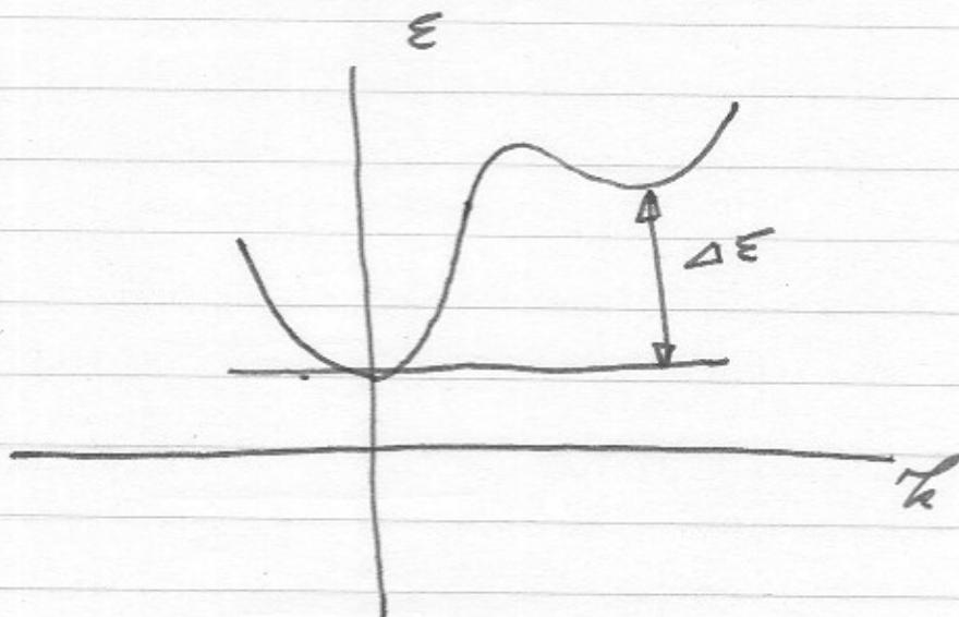
Energetic electrons in the lowest valley having kinetic energy above  $\Delta E$  the intervalley scattering, will scatter at some rate into the higher valleys. This scattering is due to phonons & is itself a random process. Once in the higher valley the electrons have much higher effective mass & lower differential mobility. They will subsequently relax to the lower valley, again at some scattering rate.
