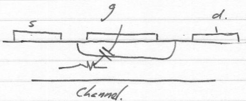
Input capacitance to device has to be charged through some portion of the channel.
