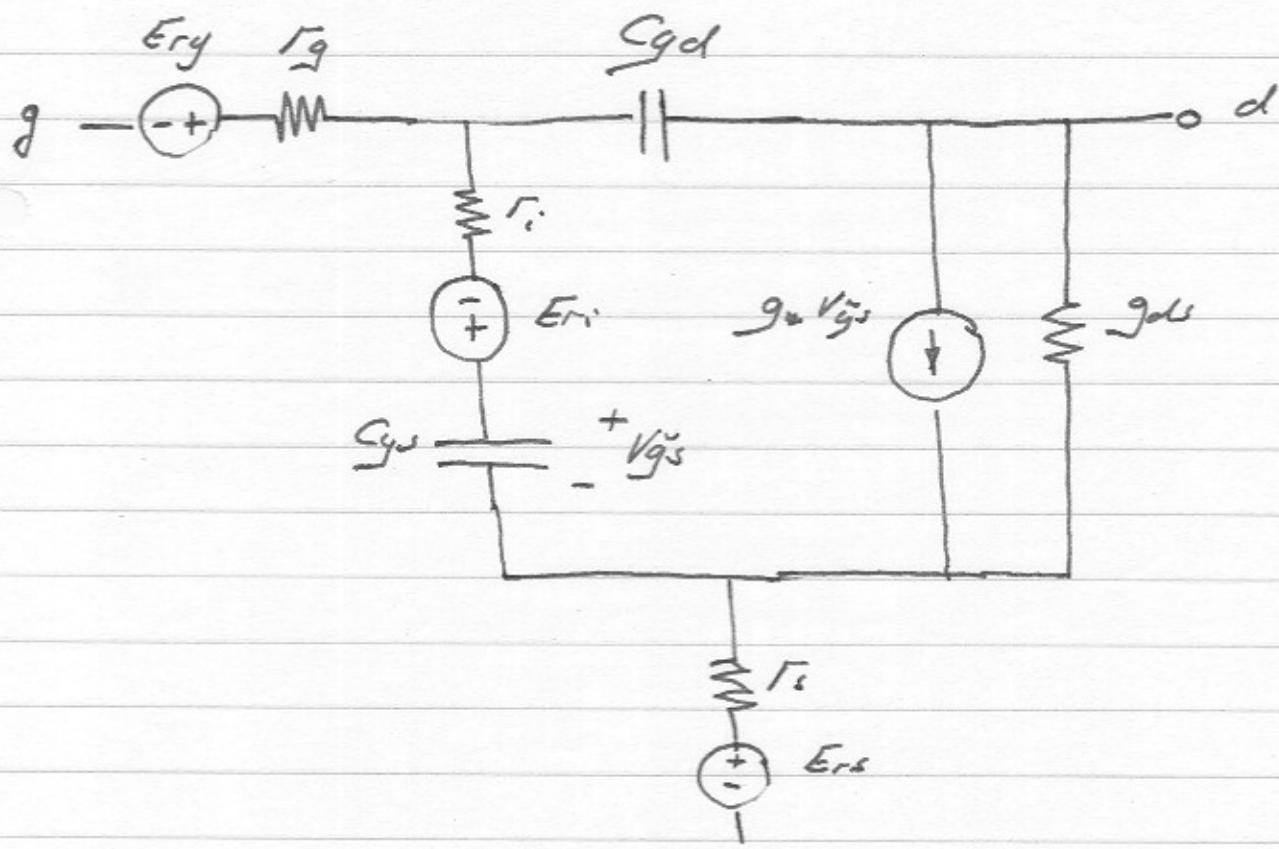
$E_{rs}$  &  $E_{rg}$  are the thermal noise of  $R_s$  &  $R_g$ ..
