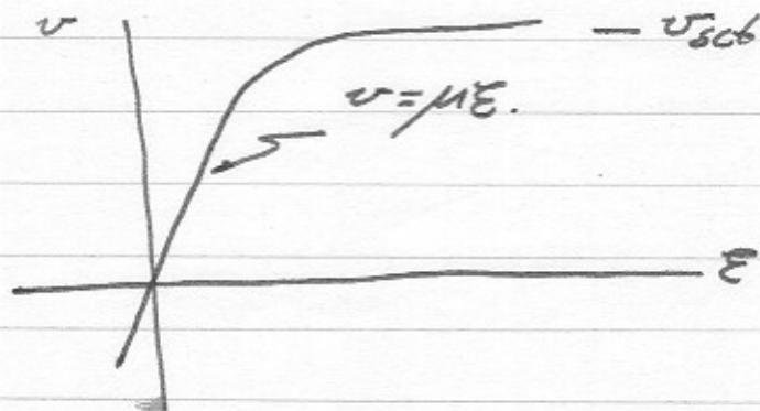
While velocity saturation is important in all semiconductor devices, the current fluctuations, hence noise, are determined by transport in low-field regions, hence we need not model the noise of high-field transport. In fets the control region itself is usually in high fields. Treatment of noise in high field regions is somewhat empirical.
