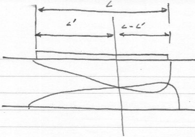
If the drain voltage is larger than the pinchoff voltage, then the drain voltage at the channel at the point of full pinch-off is  $V_o(L') = V_p$ , and the drain current is found for these conditions. Finding  $L'$  from  $V_d - V_p$  is generally difficult, involving the electrostatic problem below:
