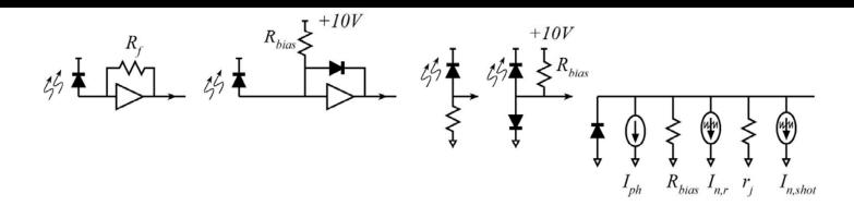
A forward - biased diode produces less noise than a resistor of equal conductance.
