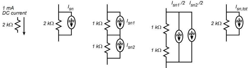
Assume: resistors have shot noise:  $\widetilde{S}_{I_{sn}I_{sn}} = 2q(1 \text{ mA})$
