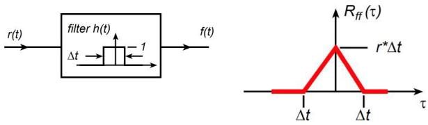
Power spectral density of  $\Delta f: S_{\Delta f \Delta f}(j\omega) = \overline{r} \cdot (\Delta t)^2 \cdot \left[ \frac{\sin(\omega \Delta t/2)}{(\omega \Delta t/2)} \right]^2$
