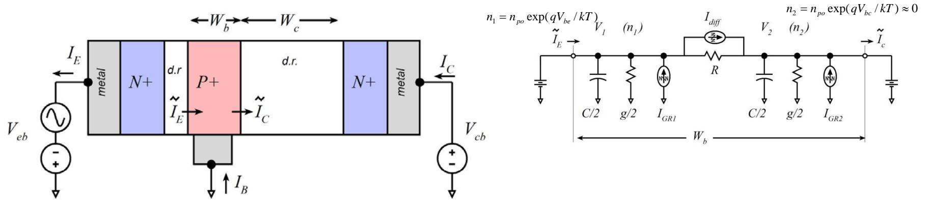
Referring to the right image (diffusion diagram), forcing  $V_{be}$  and  $V_{ce}$  forces the minority carrier concentrations  $n_1$  and  $n_2$  at the 2 edges of the base. Electron diffusion (convention) currents  $\tilde{I}_E$  and  $\tilde{I}_C$  then flow.
