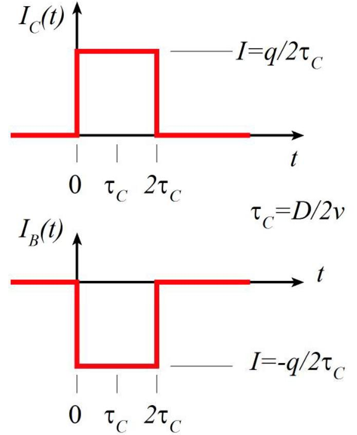
If a single electron enters the cb depletion region from the base, then the collector convection current is
