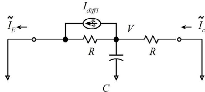
First we calculate the emitter and collector fluxes arising from  $I_{diff1}$ , noting that  $RC = \tau_b / 2$
