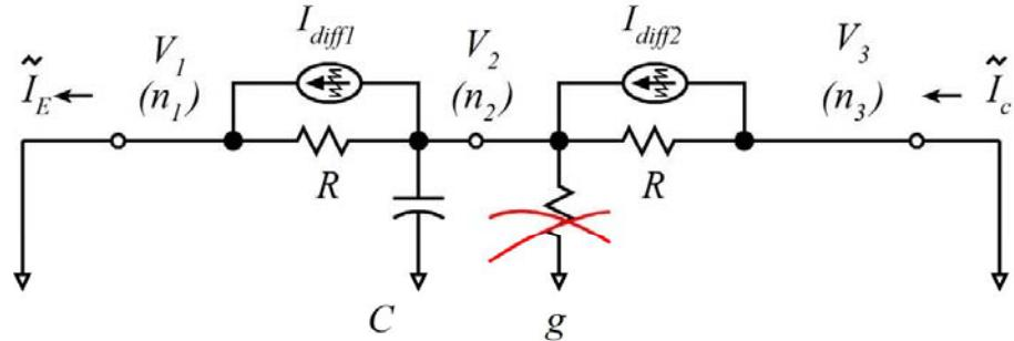
Electron densities on the 2 sides of the box of width  $W_b / 2$  are  $n_1$  and  $n_2 = n_1 / 2$ .
