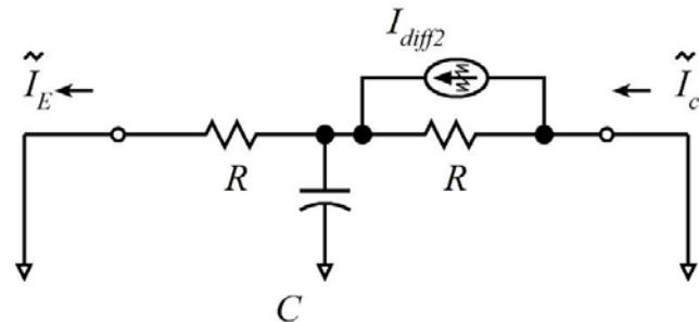
We then calculate the emitter and collector fluxes arising from  $I_{diff2}$ , noting symmetry
