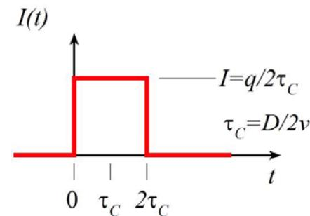
The width of this current pulse is  $D/v$ , while its mean delay (centroid) is  $\tau_c = D/2v$ .
