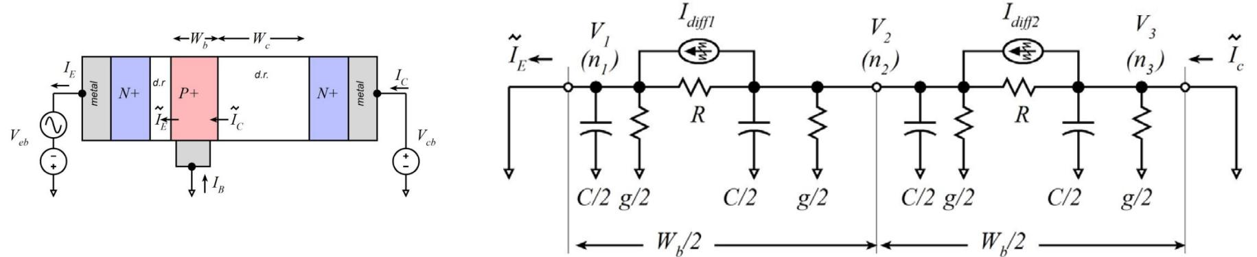
We have separated the base into 2 sections. We concentrate on diffusion noise, ignoring generation/recombination noise. Note the  $W_b / 2$  terms in the expressions arising from the finite elements of width  $W_b / 2$ .
