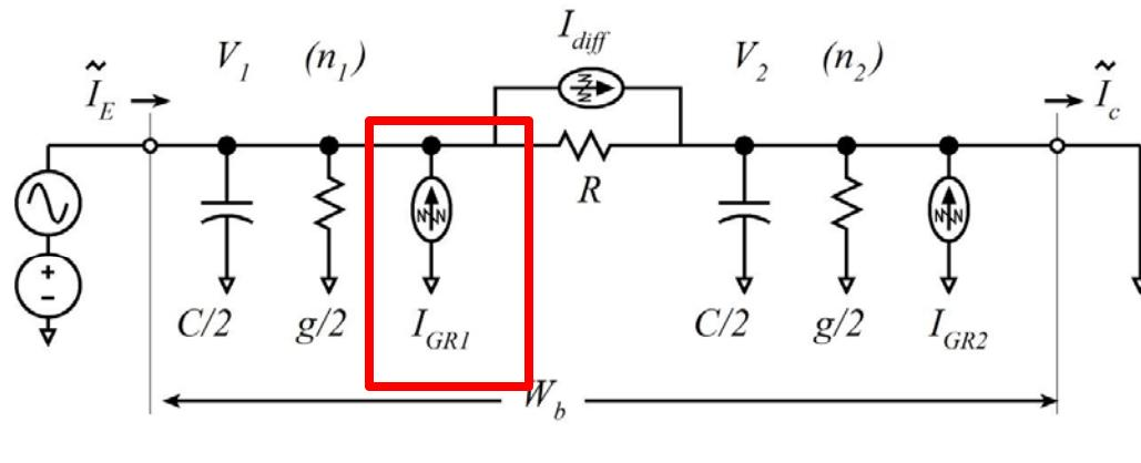
$$\begin{aligned} n_1 &= n_{po} \exp(qV_{be}/kT) & g/2 &= qAW_b/2\tau_R \\ n_2 &= n_{po} \exp(qV_{bc}/kT) \approx 0 & C/2 &= qAW_b/2 \\ R &= W_b/qAD_n \end{aligned}$$
