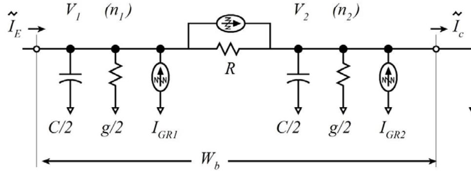
Note that  $\tilde{I}_c$  and  $\tilde{I}_E$  are the electron \* particle \* currents crossing the emitter - base and base - collector depletion regions.
