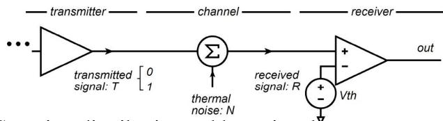
N = thermal noise, Gaussian distribution, adds to signal.
