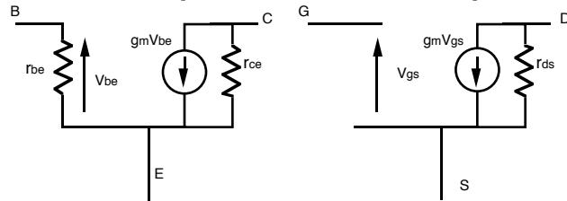
Left is the equivalent circuit of a bipolar transistor;  $g_m = I_E/V_T = 1/r_e$ ,  $V_T = kT/q$ ,  $r_{be} = \beta r_e = \beta/g_m$ . On the right is the FET model. Below is a transistor with ac equivalent load resistances  $R_C$ ,  $R_E$ , and  $R_B$ .
