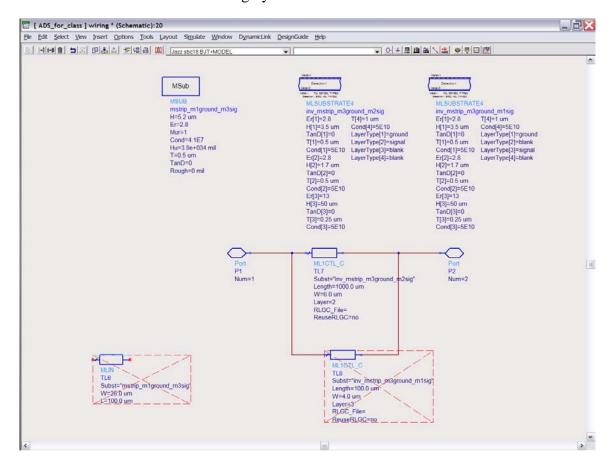
The model "inv\_mstrip\_m3ground\_m2sig" is used for lines with an M3 ground plane and M2 signal line. The model "inv\_mstrip\_m3ground\_m1sig" is used for lines with an M3 ground plane and M1 signal line. There are limitations for this modeling strategy:
