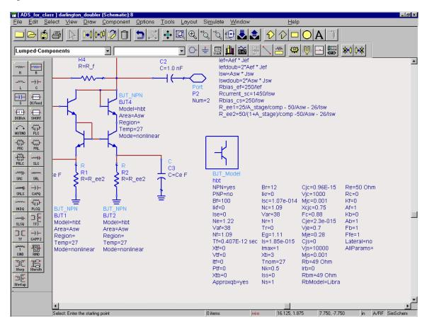
We have a model file, BJT\_MODEL, which we then invoke with an area statement. This is a large signal model which defaults to a small signal model (with bias-dependent parameters) when we do a S-parameter simulation.
