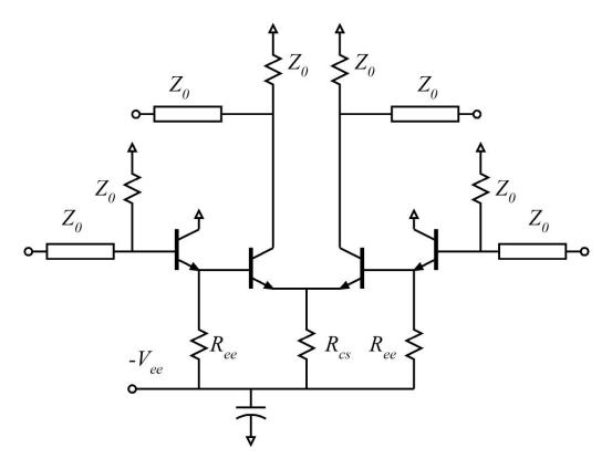
Simulate this to determine the 4 S-parameters. Determine the gain and bandwidth of S21. Recall that S-parameters are equivalent to gains with 50 Ohm generator and load impedances.
