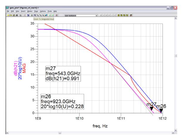
The device has an ft around 540 GHz and an fmax around 900 GHz.
