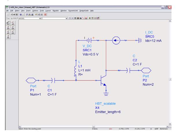
Using the above model and the biased\_HBT test bench, set up a transistor with the above parameters, but adjust the bias to a current density of 1 mA *per linear micron of emitter length* and Vcb=0.5 Volts. Simulate and plot H21 and U. Determine ft and fmax.
