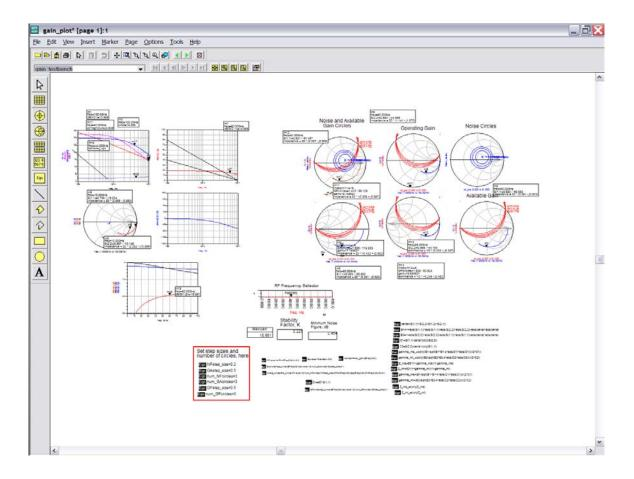
There are dB and polar plots of S-parameters, and plots of H21 and U (relevant for transistors, no relevant for the IC). There are also noise figure circles and gain circles, which are relevant to microwave tuned amplifier design.
