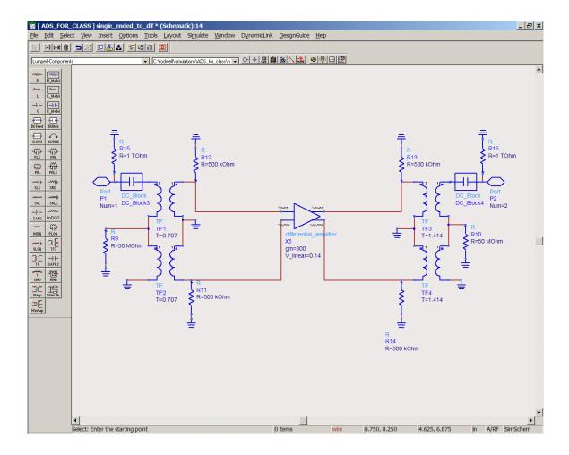
This is a utility block I created, which allows one to simulate for S parameters of a differential circuit (in this case the circuit is differential\_amplifier). This is a trick to overcome a shortcoming in ADS: it is otherwise hard to make it compute S parameters of differential circuits. Pop into it, and you see a common form of high frequency amplifier:
