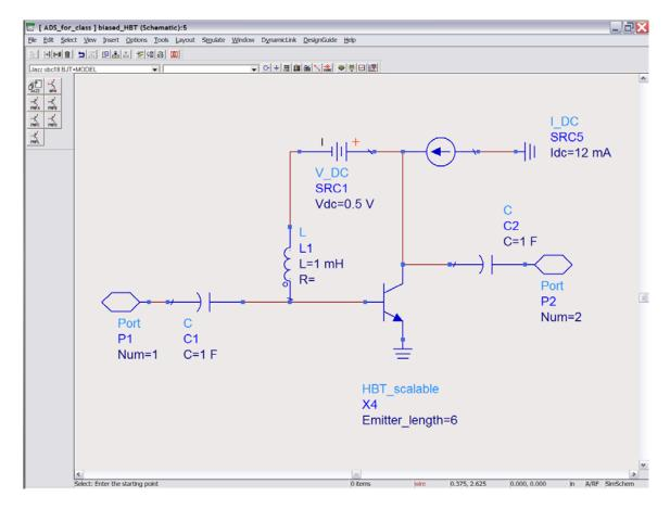
HBT\_scalable is a subcircuit with PASSED parameters
