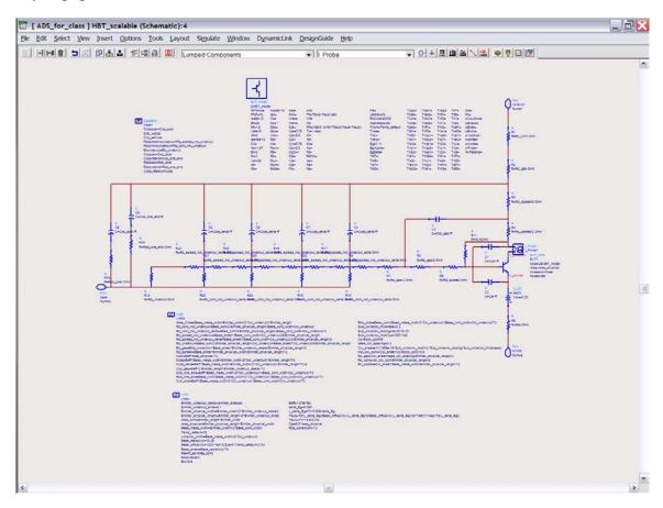
The transistor is defined as a SPICE model (DHBT model), with external parasitic resistances and capacitances which we have defined through equations from the transistor geometry. We do this at UCSB because it allows us to make fairly accurate predictions of performance of future transistors which we may not yet have built.
