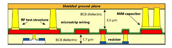
Note the thicknesses of the two BCB layers, and note that BCB has a dielectric constant of 3.8. Below the plane of the HBT subcollector, and below the resistors and metal 1, lies the semi-insulating InP substrate, having a dielectric constant of 13. We will approximate that M1 and M2 are each 1/2 micron thick.
