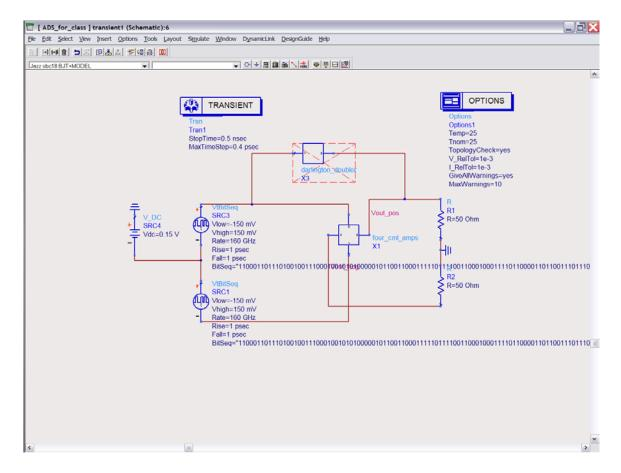
You will see a couple of circuits. Darlington\_doubler is a single-ended circuit, and is currently "inactivated". There is a differential circuit, "four\_cml\_amps", which is active. There is a pair of (random) data string generators, which are logical complements of each other. For square-wave testing you could replace these with e.g. a square wave generator.
