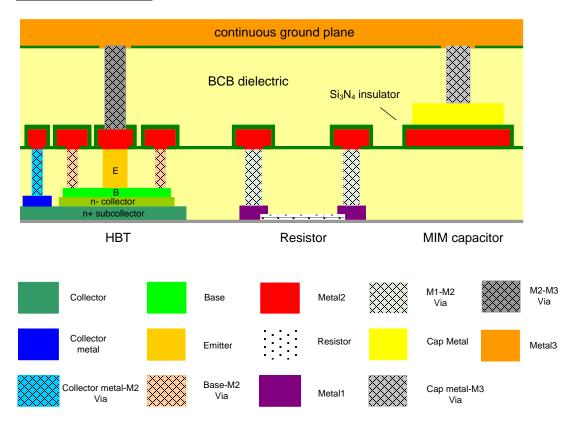
The process provides three metal layers, M1, M2, and M3. Normally, M3 will be used as a ground plane and M1 or M2 as signal lines.
