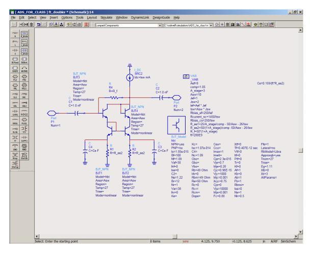
Note that a different transistor model is here used; there is no subcircuit with an associated set of equation-defined parasitics. This is the more common approach in IC design.
