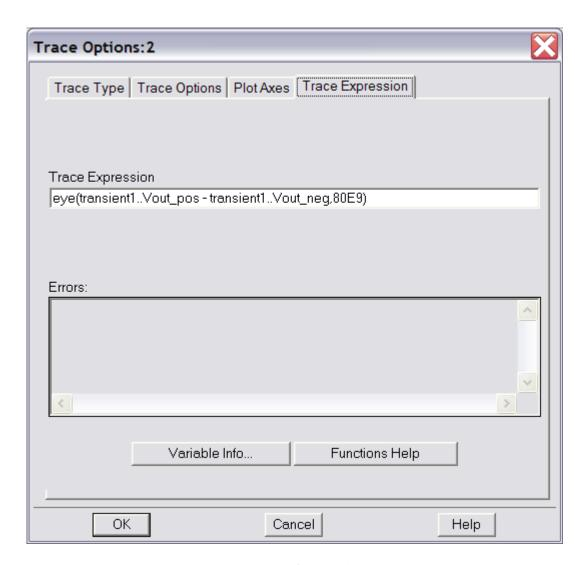
Note that the last number 80E9, is set at 1/2 the bit rate of the simulation.
