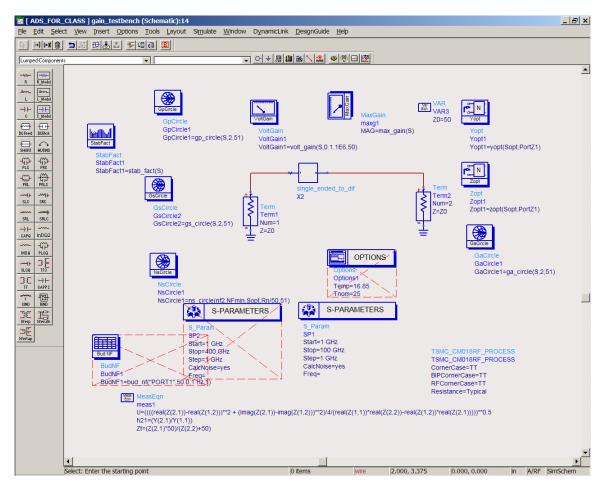
This will test for Sparameters of the subcircuit "single\_ended\_to\_dif". You can type the name of other subcircuits there to test them instead.
