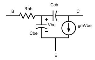
To fully work with the common-base stage, we need a slightly better model. Continue with the same assumptions and value assignments as above, except we have added Rbb. In a typical HBT, Rbb might be perhaps 10 times 1/gm and Ccb perhaps equal 1/40 of Cbe when the device is at peak bias. Lets thus set Rbb=10/gm and Ccb=0.1 Cbe. The value of Vb2 is fairly unimportant, but lets set it equal to 2.5 volts.
