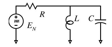
A filter of 1 Hz bandwidth, observed for 1 second, has two degrees of freedom  $(\sin(2\pi f_o) \& \cos(2\pi f_o))$ , hence the total available power in this bandwidth must be  $kT\Delta f$ .
