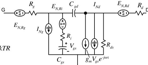
$R_g$ ,  $R_s$ ,  $R_d$  are physical resistances  $\Rightarrow d\langle V^2 \rangle / df = 4kTR$
