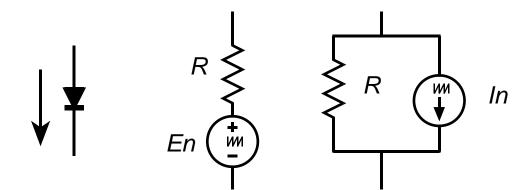
A biased diode has noise 1/2 that of a resistor of equal small - signal impedance. The factor of 2 arises from one - way current flow.
