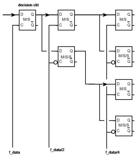
Note that M/S/S latches are required to prevent timing skew.
