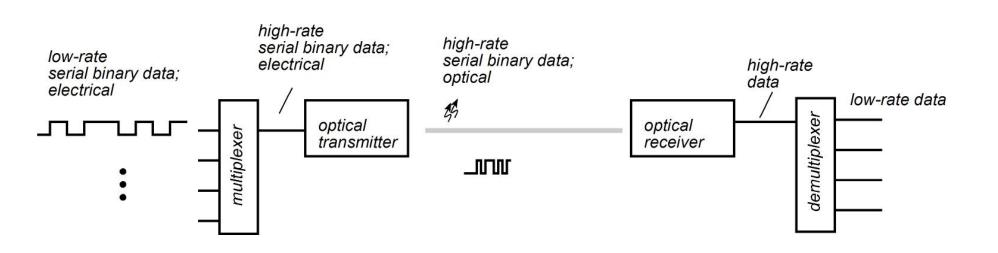
Typical form of optical link: mux, transmitter, receiver, demux
