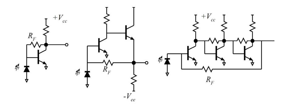
Left: low - gain, wideband design for very high bit rates.
