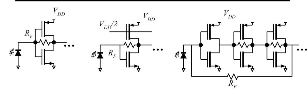
Left 2 designs are low - gain, wideband designs for very high bit rates.
