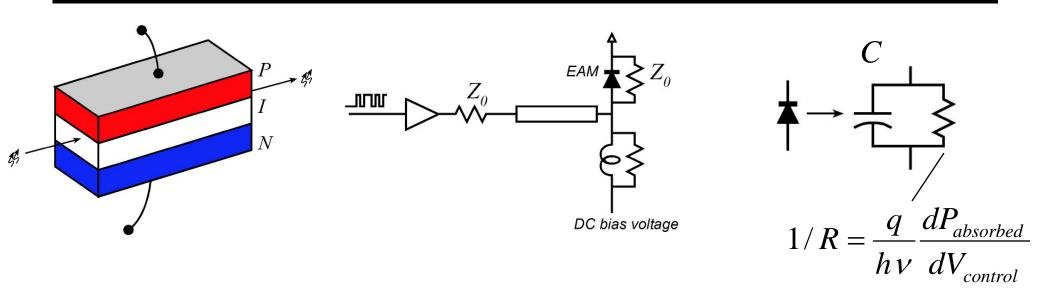
Electro - Absorbion modulators: A reverse - biased PIN junction containing an optical waveguide in the I region. Varying the reverse bias varies the optical attenuation. Electrical model is that of a reverse - biased diode, but with a parallel resistance representing the absorbed light.
