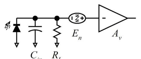
$1/2\pi f_{high} = C_{in}R_L$  (need smaller *R* for same bandwidth)
