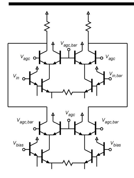
Upper half is basic AGC cell: Differential pair with variable current shunt.
