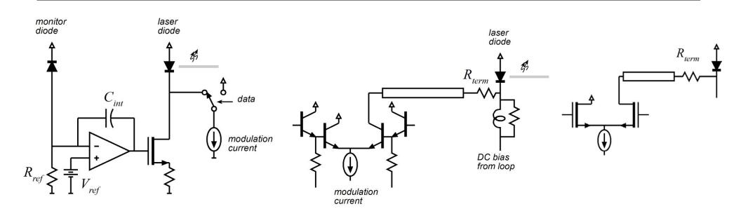
Basic Form; sometimes uses DC feedback loop to maintain laser bias.
