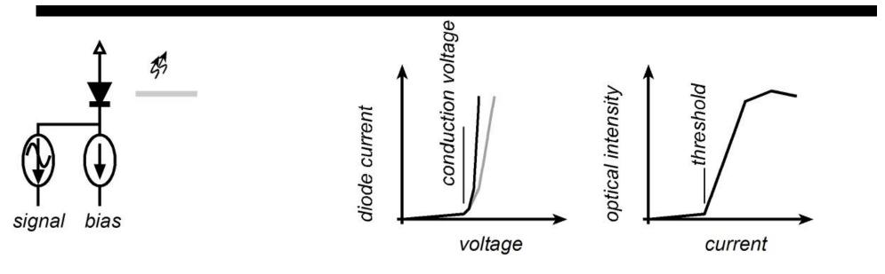
Diode is driven by superposition of bias and AC drive current.
