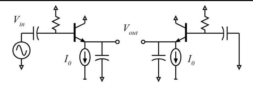
DC currents in the 2 BJTs are forced by current sources all to be  $I_0$ . Analysis (work in lecture) shows that for a inputs much larger than kT/q,  $V_{out} = V_{in,peak-peak} / 2 - kT / q - I_o T_{bit} / C$
