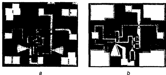
Fig. 2 IC chip photographs of mirror doubler amplifier and high gain Darlington amplifier
