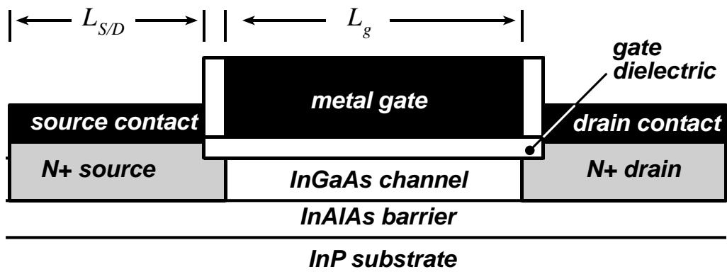
Predicted drive current:  $\sim 5 \text{ mA}/\mu\text{m}^{1,2}$
