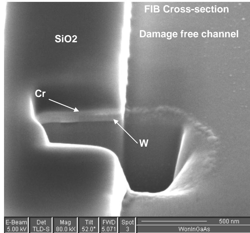
*Process scalable to sub-100 nm gate lengths*
