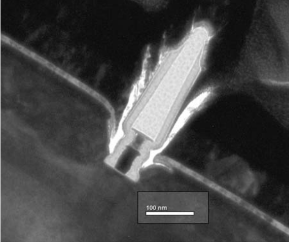
Figure 7: Cross-section of regrown S/D InGaAs FET with a 27 nm gate
