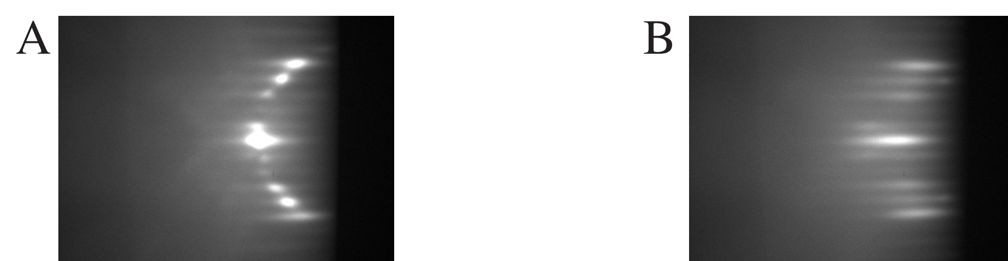
Figure 6: Representative RHEED images of InAs regrowth (A) at the beginning of the regrowth and (B) at the end of the regrowth.
