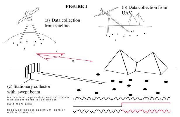
The nodes are capable of sensing any given phenomenon of interest, and we employ an imaging approach to data collection. A sophisticated, location-aware, collector node scans the sensor field systematically using a radio frequency (RF) beacon. Sensor nodes being scanned ``reflect" the beacon (possibly also modulating it with low rate data) either actively
