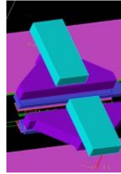
Figure 4.3: Transistor layout up to top metal layer in electromagnetic simulation environment
