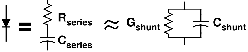
Figure 2.7: A diode is modeled as a series RC network. This series network has an equivalent shunt network, with different component values.
