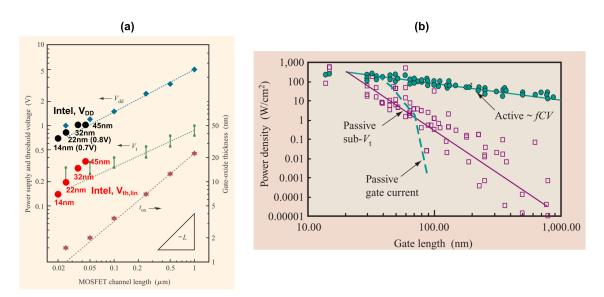
Figure 1.1: (a)  $V_{\text{DD}}$  scaling,  $V_{\text{th}}$  scaling, and the oxide thickness scaling for the previous CMOS generations (Modified figure from [2]). (b) Active power consumption and standby power consumption as a function of gate lengths [3].
