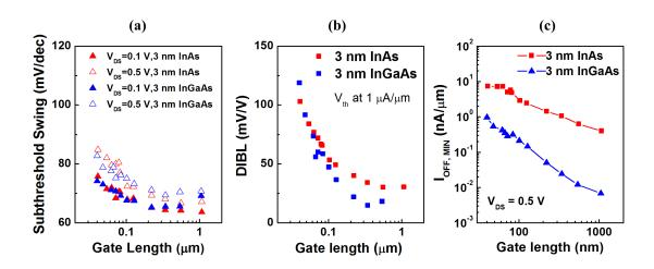
Figure 4.9: (a) Subthreshold swing vs.  $L_{\rm g}$ . (b) DIBL vs.  $L_{\rm g}$ . (c)  $I_{\rm off,min}$  vs.  $L_{\rm g}$  at  $V_{DS}$ =0.5 V.
