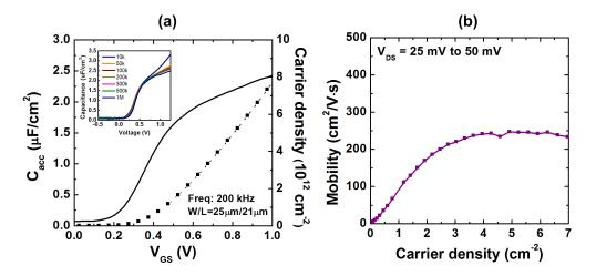
Figure 6.7: (a) Capacitance-voltage measurements for 2.5 nm composite channel MOSFETs. The inset shows C-V frequency dispersion. (b) The extracted effective channel mobility using split C-V measurements for 25  $\mu$ m- $L_{\rm g}$  devices.
