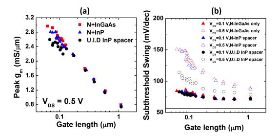
Figure 5.4: (a) Comparison of  $g_{\rm m}$  versus  $L_{\rm g}$  for samples 5.2A, 5.2B, and 5.2C. (b) Comparison of SS versus  $L_{\rm g}$  for samples 5.2A, 5.2B, and 5.2C.
