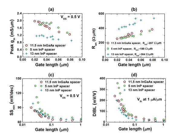
Figure 5.12: Comparisons of (a)  $g_{\rm m}$  vs.  $L_{\rm g}$ , (b)  $R_{\rm on}$  vs.  $L_{\rm g}$ , (c) SS vs.  $L_{\rm g}$ , (d) DIBL vs.  $L_{\rm g}$  for 4.5 nm InGaAs channel MOSFETs with a 5 nm recessed InP spacer (sample 5.4A), a 13 nm recessed InP spacer (sample 5.3B), and a 11.5 nm InGaAs spacer (sample 5.3A).
