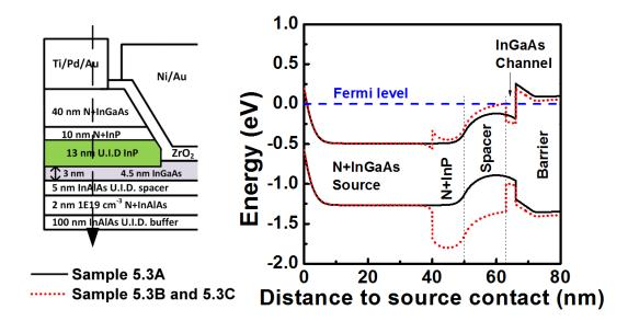
Figure 5.9: Energy band diagrams of the three samples, drawn on a path passing through the N+source and into the channel and the barrier.
