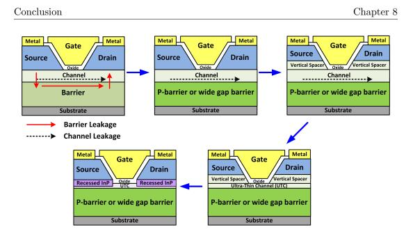
Figure 8.1: Progression of III-V MOSFET designs for reduced off-state leakage.
