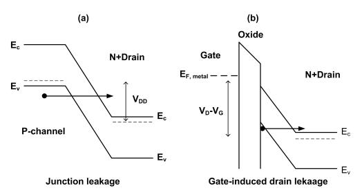
Figure 2.7: (a) The band profile of drain-to-channel junction under reverse bias. (b) The band profile at the gate-drain overlap region at large negative  $V_G$  and positive  $V_D$ .
