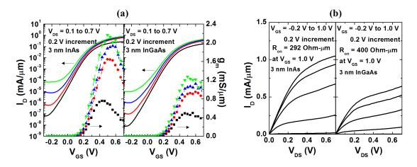
Figure 4.7: (a) The transfer characteristics and (b) the output characteristics of  $L_{\rm g}$ -40 nm devices.
