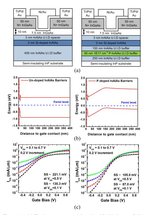
Figure 3.12: (a) The device structures with un-doped InAlAs barriers (left) and P-doped InAlAs barriers (right). (b) The corresponding band energy diagrams. (c) The corresponding  $I_{\rm DS}$ - $V_{\rm GS}$  curves of 50 nm- $L_{\rm g}$  devices.
