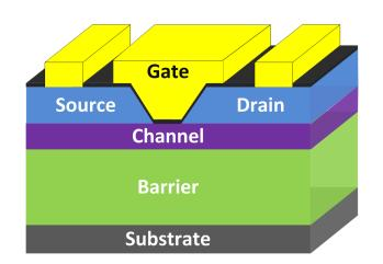
Figure 1.3: UCSB ultra-thin channel planar MOSFETs.
