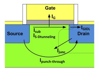
Figure 2.6: The possible leakage paths in nanoscale MOSFETs.
