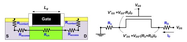
Figure 2.4: (a) The series resistance in MOSFETs. (b) The circuit diagram of MOSFETs with series resistance.
