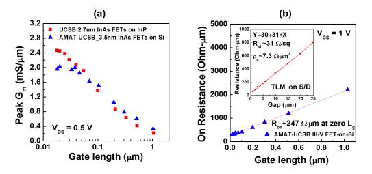
Figure 7.5: (a) Comparison of  $g_{\rm m}$  and (b)  $R_{\rm on}$  as a function of  $L_{\rm g}$  for this work on Si substrates and 2.7 nm InAs MOSFETs on InP.
