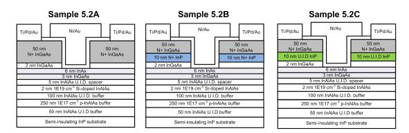
Figure 5.1: Device structures of sample 5.2A with N+InGaAs source/drain, sample 5.2B with N+InP source/drain, and sample 5.2C with 10 nm undoped InP source/drain spacers.
