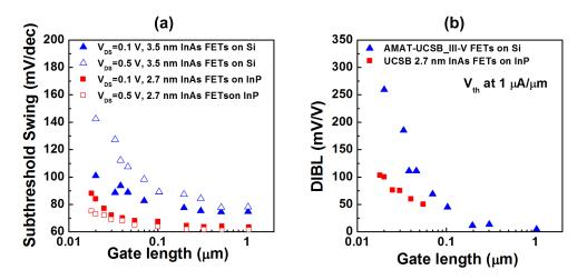
Figure 7.6: (a) Comparison of SS and (b) DIBL as a function of  $L_{\rm g}$  for this work on Si substrates and 2.7 nm InAs MOSFETs on InP.
