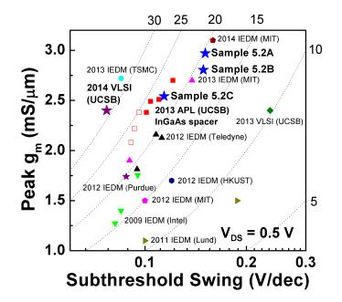
Figure 5.5: Benchmark of  $g_{\rm m}$  and SS for the three samples in this section to recently reported III-V MOSFETs.
