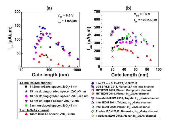
Figure 5.17: (a)  $I_{\rm on}$  vs.  $L_{\rm g}$  at  $I_{\rm off}=1$  nA/ $\mu$ m and  $V_{\rm DS}=0.5$  V. (b)  $I_{\rm on}$  vs.  $L_{\rm g}$  at  $I_{\rm off}=100$  nA/ $\mu$ m and  $V_{\rm DS}=0.5$  V and the benchmark with recently published III-V MOSFETs.
