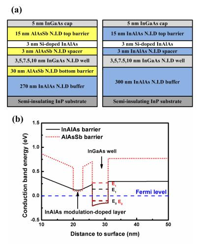
Figure 3.2: (a) The InGaAs/AlAsSb and InGaAs/InAlAs 2DEG quantum well layer structures using modulation-doped InAlAs layers above the well. (b) Simulated conduction band profile for a 5 nm InGaAs well. The dashed lines indicate the Fermi level and the first two bound states band minima within the well.
