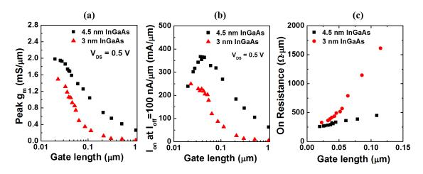
Figure 4.13: (a) The transconductance, (b) on-state current at 100 nA/ $\mu$ m  $I_{\text{off}}$ , and (c) on-resistance as a function of gate length for 4.5 nm InGaAs and 3 nm InGaAs MOSFETs.
