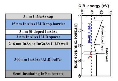
Figure 4.3: Double heterostuctures for the study of electron transport in quantum wells and the associated band diagram calculated by 1-D self-consistent Schrödinger-Poisson simulation.
