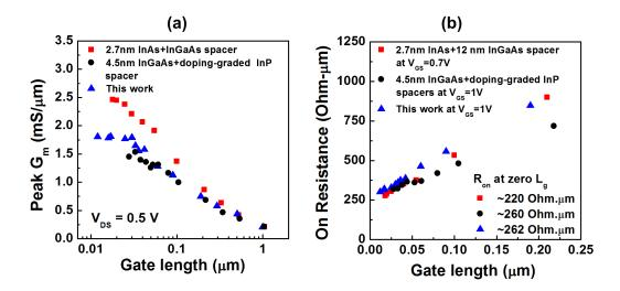
Figure 6.4: (a) Comparison of  $g_{\rm m}$  and (b)  $R_{\rm on}$  as a function of  $L_{\rm g}$  for 2.5 nm composite channels MOSFETs to previously reported high performance InAs MOSFETs (chapter 4.4 and [10]) and low leakage InGaAs MOSFETs with recessed InP spacers (chapter 5.5 and [11])
