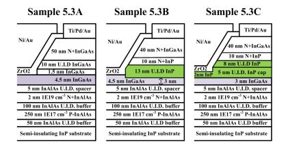
Figure 5.6: Devices structures of sample 5.3A (raised InGaAs spacer), 5.3B (recessed InP spacer), and 5.3C (InP cap layer). The devices have symmetric source/drain and only the drain side of the devices is shown here.
