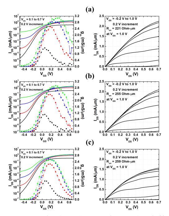
Figure 5.2: Transfer and output characteristics of  $L_g=65$  nm devices for (a) sample 5.2A, (b) sample 5.2B, and (c) sample 5.2C.
