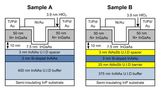
Figure 3.7: Device structure of sample A(In<sub>0.52</sub>Al<sub>0.48</sub>As barrier) and sample B (AlAs<sub>0.56</sub>Sb<sub>0.44</sub> barrier). The pulse doping layer is 3 nm,  $1.3 \times 10^{19}$  cm<sup>-3</sup> Si-doped In<sub>0.52</sub>Al<sub>0.48</sub>As. The InGaAs channel thickness is 7.5 nm. (U.I.D. = un-intentionally doped)
