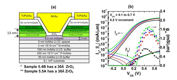
Figure 5.13: (a) The device schematic diagram of the InGaAs MOSFET with a recessed, doping graded InP spacer. (b) The transfer characteristic of sample 5.4B at  $L_{\rm g}$ -30 nm, having a 30 Å ZrO<sub>2</sub>.
