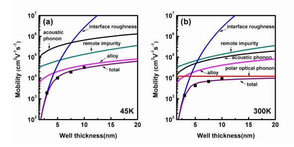
Figure 3.4: Measured and calculated (a) low temperature (45 K) and (b) room temperature (300 K) Hall mobilities of InGaAs/AlAsSb 2DEGs as a function of InGaAs quantum well thickness.
