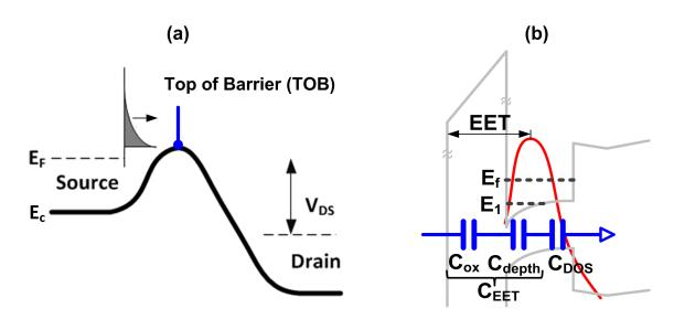
Figure 2.1: (a) The band diagram of MOSFETs along the channels, showing that the position of top-of-barrier determines the amount of current flow from the source to the drain. (b) The gate-to-channel capacitance consists three series capacitances, including oxide capacitance, wave-function depth capacitance, and density-of-state capacitance (Courtesy of Sanghoon Lee).
