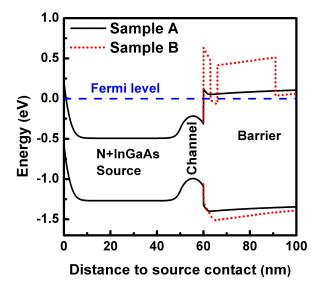
Figure 3.11: Energy band diagram of sample A ( $In_{0.52}Al_{0.48}As$  barrier) and sample B ( $AlAs_{0.56}Sb_{0.44}$  barrier) with raised N+ InGaAs source/drain (Sidoped:  $4 \times 10^{19}$  cm<sup>-3</sup>), drawn on a vertical line passing through the N+ source, the InGaAs channel, and the InAlAs or AlAsSb bottom barrier. Given the high source doping, the InAlAs barrier energy lies only ~ 0.1-0.2 eV above the Fermi energy, while the AlAsSb barrier provides ~ 0.6-0.7 eV carrier confinement.
