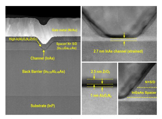
Figure 4.17: The cross-sectional STEM images of 25 nm- $L_g$  InAs MOSFETs, showing ~2.7 nm InAs channel, ~1 nm AlO<sub>x</sub>N<sub>1-x</sub> interfacial layer and ~2.5 nm ZrO<sub>2</sub> gate dielectric. The source/drain has ~12 nm un-doped InGaAs vertical spacer and the N+InGaAs contact layers.(Courtesy of Sanghoon Lee)
