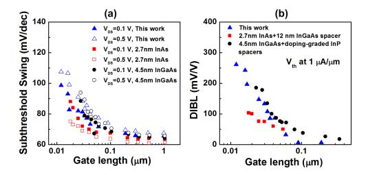
Figure 6.5: (a) Comparison of SS and (b) DIBL as a function of  $L_{\rm g}$  for 2.5 nm composite channels MOSFETs to previously reported high performance InAs MOSFETs (chapter 4.4 and [10]) and low leakage InGaAs MOSFETs with recessed InP spacers (chapter 5.5 and [11])
