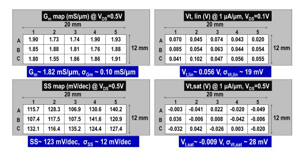
Figure 7.8: The maps of  $g_{\rm m}$ , SS,  $V_{t,lin}$ ,  $V_{t,sat}$  for 45 nm- $L_{\rm g}$  devices on the 2 mm×1.2 mm samples.
