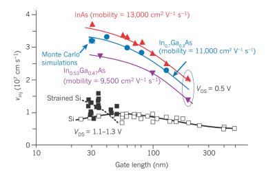
Figure 1.2: Comparison of electron injection velocity of III-V HEMT and Si MOSFETs [7].
