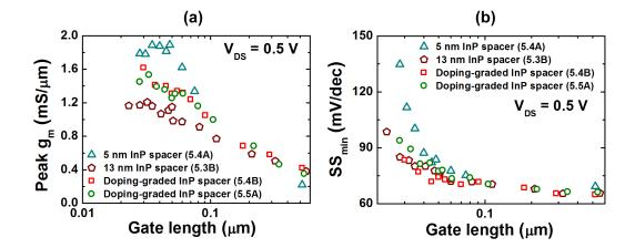
Figure 5.16: Comparisons of (a)  $g_{\rm m}$  vs.  $L_{\rm g}$  and (b) SS vs.  $L_{\rm g}$  for a doping– graded InP spacer, a 5 nm undoped InP spacer, and a 13 nm undoped InP spacer.
