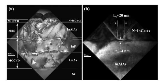
Figure 7.2: (a) A TEM image of the whole device structure, showing Applied Material III-V buffers on Si, UCSB MBE grown back barriers and the InAs/InGaAs channels with  $ZrO_2$  high-k/Ni metal gate, and UCSB MOCVD InGaAs source/drain regrowth. (b) The magnified TEM image on the channel regions of a 20 nm- $L_g$  device.
