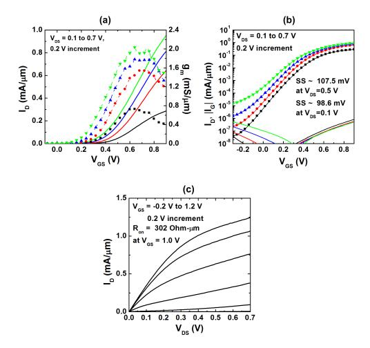
Figure 6.3: (a)  $I_{\rm D}$  and transconductance  $g_{\rm m}$  versus  $V_{\rm GS}$ , (b) subthreshold characteristics, and (c) output characteristics for a 12 nm- $L_{\rm g}$  FET.
