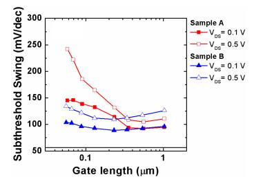
Figure 3.10: Subthreshold swing vs.  $L_{\rm g}$  for sample A and sample B at  $V_{\rm DS}{=}0.1$  V and  $V_{\rm DS}{=}0.5$  V.
