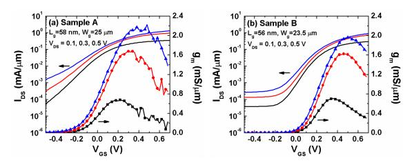
Figure 3.8: Transfer characteristics of (a) sample A with  $L_g=56$  nm and (b) sample B with  $L_g=58$  nm at  $V_{\rm DS}$  of 0.1, 0.3, and 0.5 V.
