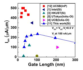
Figure 7.7:  $I_{\text{on}}$  at fixed  $I_{\text{off}}=100 \text{ nA}/\mu\text{m}$  for recently reported planar III-V FETs on Si [1,3–5,11], and compared to results on InP [12].
