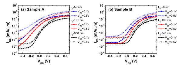
Figure 3.9: Subthreshold characteristics (a) of sample A with  $L_g=56$ , 131, and 558 nm and (b) of sample B with  $L_g=58$ , 130, and 540 nm.
