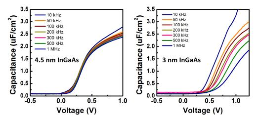
Figure 4.14: The capacitance-voltage measurements of  $L_{\rm g}$ -25  $\mu$ m MOSFETs for 4.5 nm and 3 nm InGaAs channels and ZrO<sub>2</sub> gate dielectrics. The source and drain are grounded and the measured frequency varies from 10 kHz to 1 MHz.
