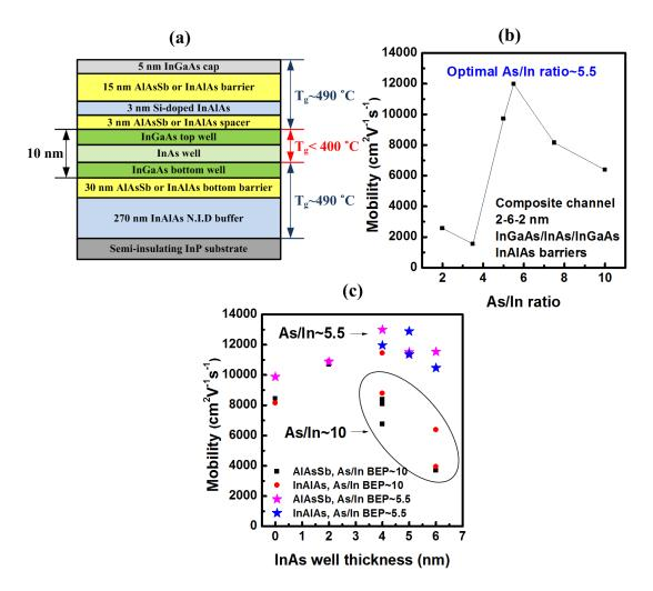
Figure 4.2: (a) The composite channel 2DEG structures and the respective growth temperature for each layer. (b)The dependency of 2DEG mobility for 2-6-2 nm InGaAs-InAs-InGaAs composite channels on the As/In BEP ratio during the 6 nm InAs growth. (c) Composite channel 2DEG mobility as a function of the InAs well thickness.(The channels are 10 nm InGaAs, 4-2-4 nm, 3-4-3 nm, 2.5-5-2.5 nm, and 2-6-2 nm InGaAs-InAs-InGaAs composite channels.)
