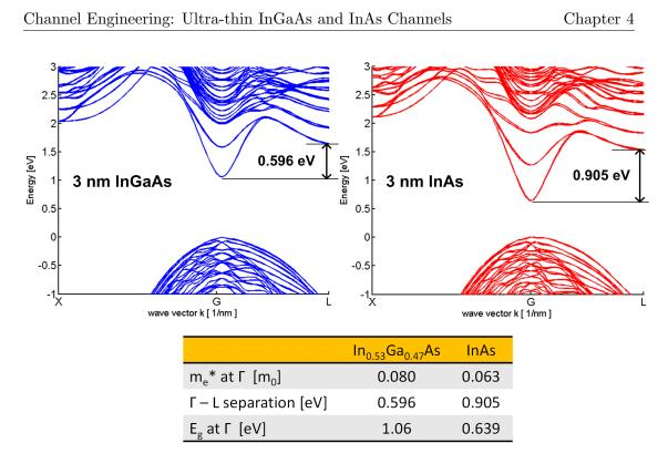
Figure 4.10: Tight binding band structures of 3 nm InGaAs and 3nm InAs wells with a hydrogen-terminated top surface and 2 nm InAlAs bottom barriers. No strain effect on InAs channel is considered in the calculations.
