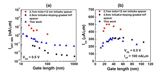
Figure 6.6: (a) Comparison of minimum  $I_{\text{off}}$  at  $V_{\text{DS}}=0.5$  V and (b)  $I_{\text{on}}$  at fixed  $I_{\text{off}}=100$  nA/ $\mu$ m and  $V_{\text{DS}}=0.5$  V as a function of  $L_{\text{g}}$  for 2.5 nm composite channels MOSFETs to previously reported high performance InAs MOSFETs (chapter 4.4 and [10]) and low leakage InGaAs MOSFETs with recessed InP spacers (chapter 5.5 and [11])
