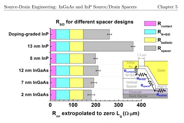
Figure 5.14: Comparison of the parasitic source/drain resistance with respect to different spacer designs.
