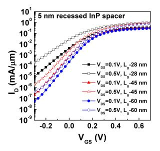
Figure 5.11:  $I_{\rm D}$ - $V_{\rm GS}$  characteristics vs.  $L_{\rm g}$  for InGaAs FETs with 5 nm recessed InP spacers.
