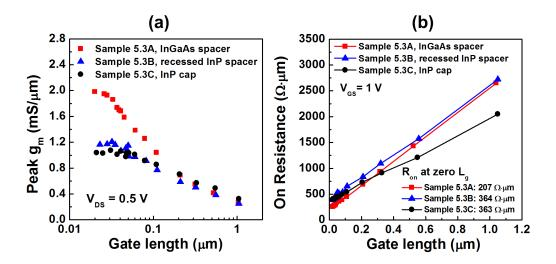
Figure 5.8: Comparison of (a)  $g_{\rm m}$  versus  $L_{\rm g}$  and (b)  $R_{\rm on}$  versus  $L_{\rm g}$  for sample 5.3A, 5.3B, and 5.3C.
