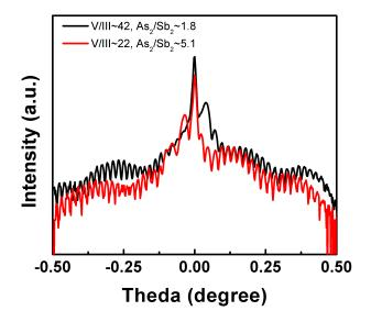
Figure 3.1: X-ray diffraction of n-doped  $AlAs_{0.56}Sb_{0.44}$  layers grown at different V/III ratio. The beam equivalent pressure ratio of  $As_2$  to  $Sb_2$  is around 5.1 for the total  $(As_2+Sb_2)/Al$  ratio~22 and  $As_2/Sb_2\sim1.8$  for total  $(As_2+Sb_2)/Al\sim42$ .
