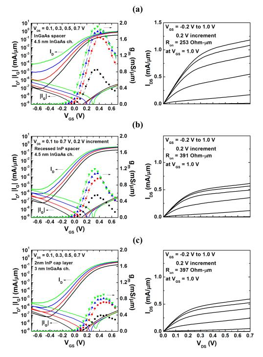
Figure 5.7: Transfer and output characteristics for (a) sample 5.3A, (b) sample 5.3B, and (c) sample 5.3C.
