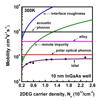
Figure 3.6: The measured and the calculated room temperature mobilities of InGaAs/AlAsSb 2DEGs as a function of 2DEG carrier concentration  $(N_s)$ . The modulation-doped impurity concentration was varied from  $1.0 \times 10^{12}$  to  $3.9 \times 10^{12}$  cm<sup>-2</sup> by controlling the Si shutter opening time or the Si cell temperature. The calculation assumes the modulation-doped impurity concentration, Ni, is  $2 \times 10^{12}$  cm<sup>-2</sup>.
