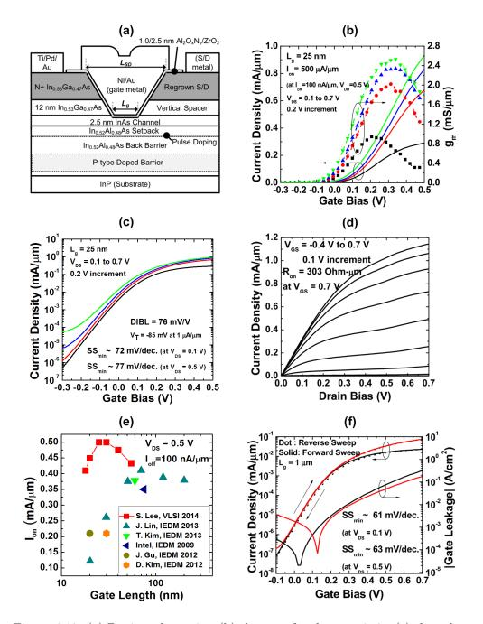
Figure 4.18: (a) Device schematics, (b) the transfer characteristic, (c) the subthreshold characteristic, and (d) the output characteristic of a 25 nm- $L_{\rm g}$  InAs MOSFET. (e) Benchmark of  $I_{\rm on}$  at fixed  $I_{\rm off}$ =100 nA/ $\mu$ m to recent published III-V MOSFETs. (f) The subthreshold characteristics of  $L_{\rm g}$ -1  $\mu$ m device, showing SS=61 mV/dec.(Courtesy of Sanghoon Lee)
