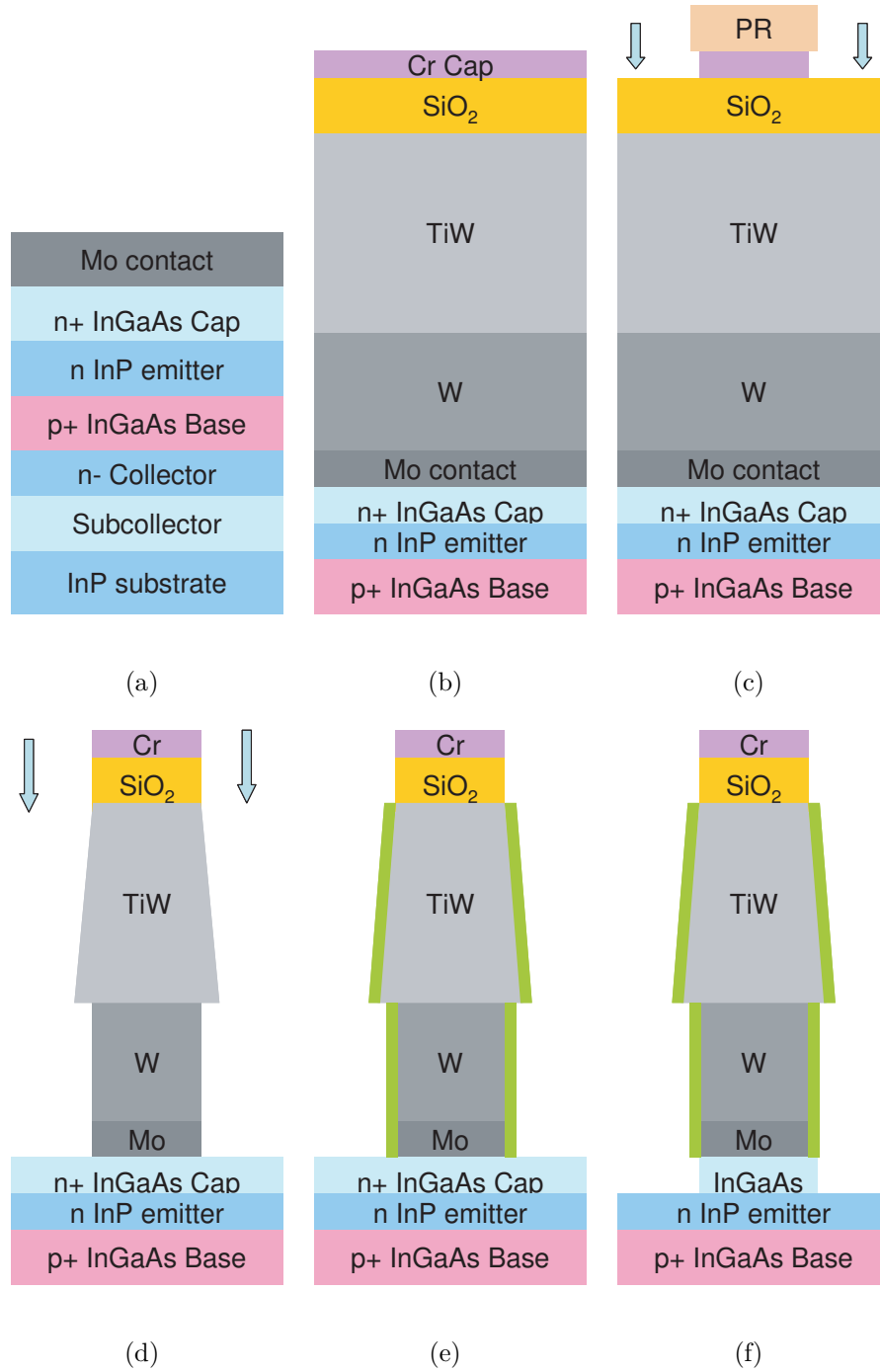
Figure 3.25: Schematic of the DHBT process flow for emitter formation - I
