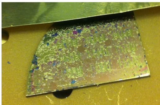
Figure 3.13: ZEP resist damaged by electron and x-ray radiation during electron beam evaporation. (a) photograph of a sample immediately after evaporation showing resist blistering, (b) low magnification SEM of a sample after stripping blistered resist.
