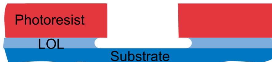
Figure 3.20: Cross-section of photoresist and LOL after exposure and development
