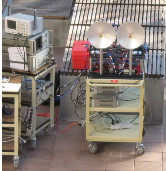
Figure 4.4: Outdoor receiver prototype
