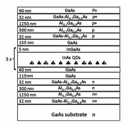
Fig. 1. Detailed structure of the samples used in the measurements,  $Al_{0.7}Ga_{0.3}As$  layers at the GaAs interfaces are graded.
